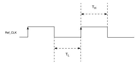
Figure 49. Reference Clock Timing Waveform
