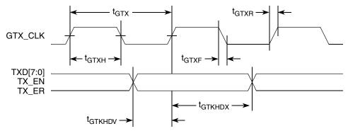
Figure 16. GMII Transmit AC Timing Diagram
