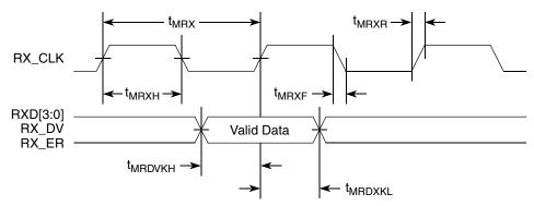
Figure 21. MII Receive AC Timing Diagram
