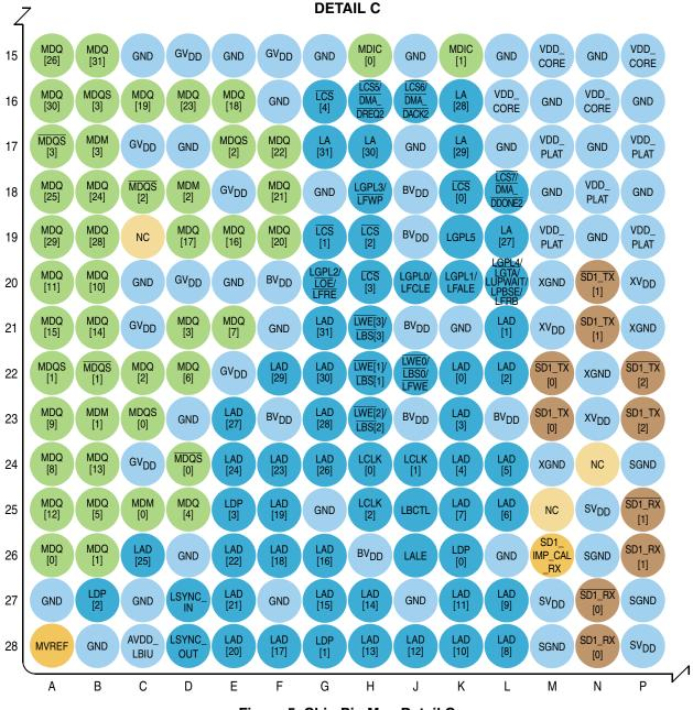
Figure 5. Chip Pin Map Detail C
