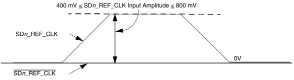
Figure 61. Single-Ended Reference Clock Input DC Requirements
