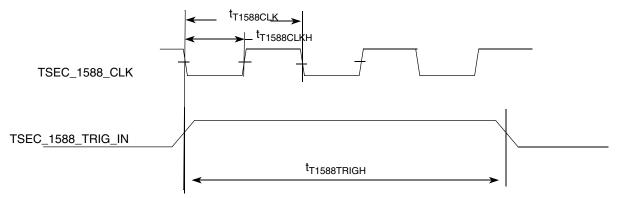
Figure 34. eTSEC IEEE 1588 Input AC timing
