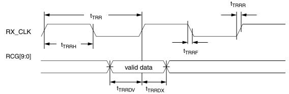
Figure 24. TBI Single-Clock Mode Receive AC Timing Diagram
