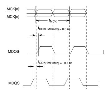
Figure 9. Timing Diagram for tDDKHMH
