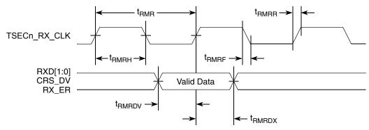
Figure 28. RMII Receive AC Timing Diagram
