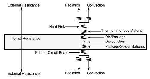
(Note the internal versus external package resistance)
