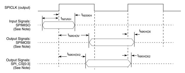
Note: The clock edge is selectable on SPI.
