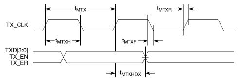
Figure 19. MII Transmit AC Timing Diagram
