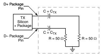
Figure 32. SGMII AC Test/Measurement Load
