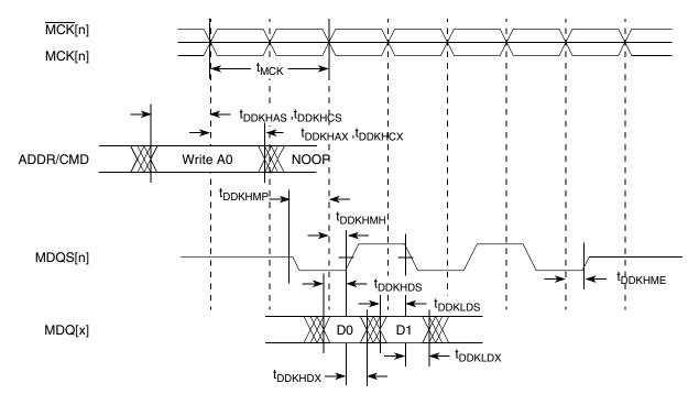
Figure 10. DDR SDRAM Output Timing Diagram
