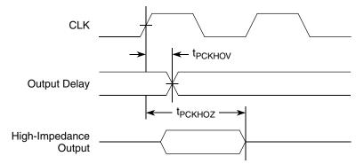
Figure 56. PCI Output AC Timing Measurement Condition
