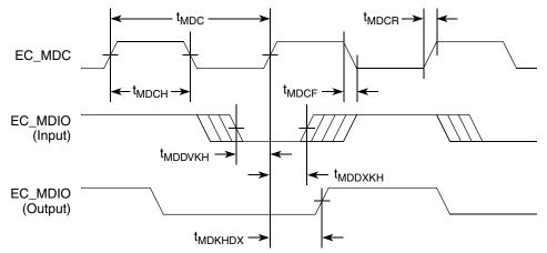
Figure 35. MII Management Interface Timing Diagram
