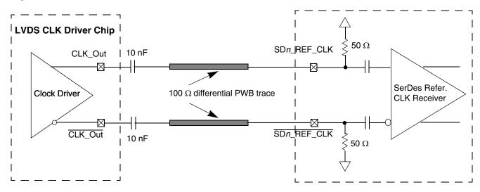
Figure 63. AC-Coupled Differential Connection with LVDS Clock Driver (Reference Only)
