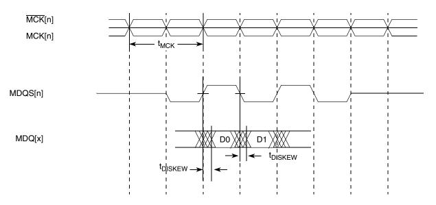
Figure 8. DDR SDRAM Input Timing Diagram
