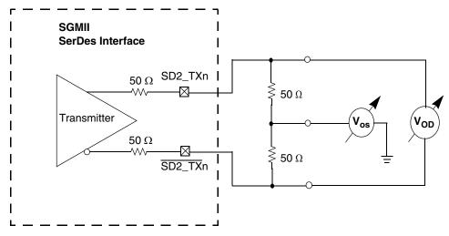
Figure 30. SGMII Transmitter DC Measurement Circuit
