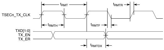
Figure 26. RMII Transmit AC Timing Diagram
