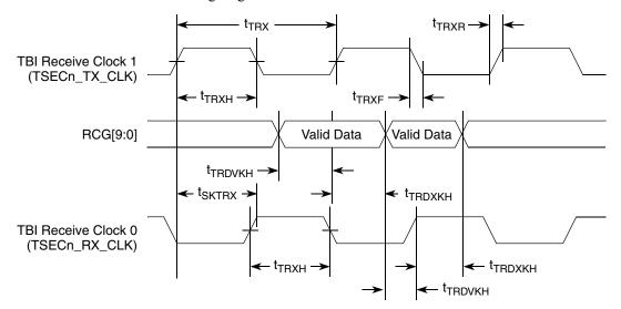
Figure 23. TBI Receive AC Timing Diagram
