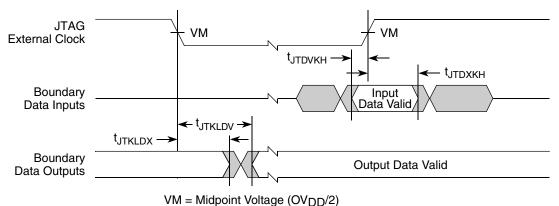
Figure 48. Boundary-Scan Timing Diagram
