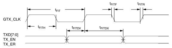
Figure 14. FIFO Transmit AC Timing Diagram
