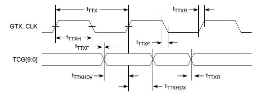
Figure 22. TBI Transmit AC Timing Diagram
