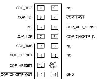
Figure 79. COP Connector Physical Pinout
