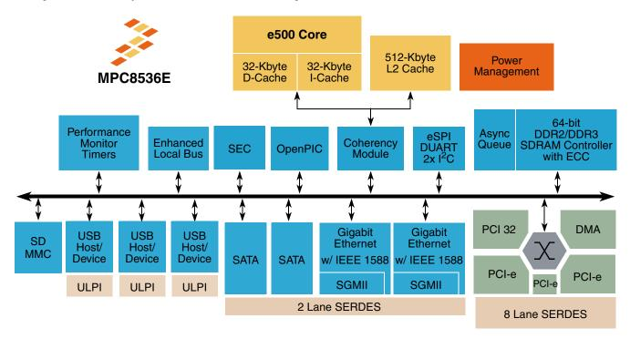
Figure 1. Chip Block Diagram
