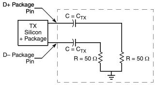
Figure 71. Compliance Test/Measurement Load
