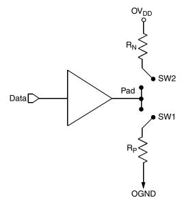
Figure 77. Driver Impedance Measurement
