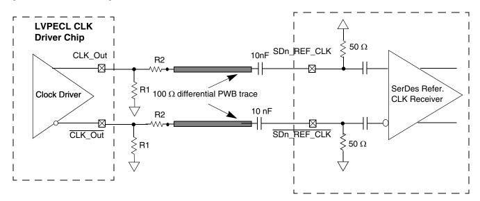
Figure 64. AC-Coupled Differential Connection with LVPECL Clock Driver (Reference Only)
