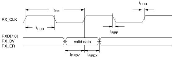
Figure 15. FIFO Receive AC Timing Diagram
