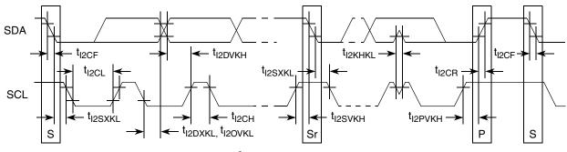
Figure 52. I<sup>2</sup>C Bus AC Timing Diagram
