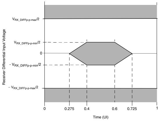
Figure 31. SGMII Receiver Input Compliance Mask
