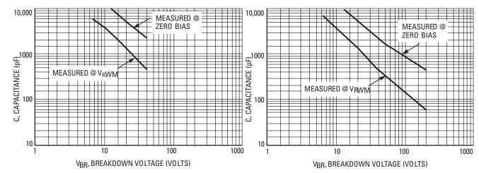
Figure 3. Capacitance versus Breakdown Voltage
