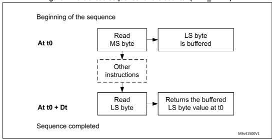
Figure 1. 16-bit read sequence for the counter (TIMx\_CNTR)
