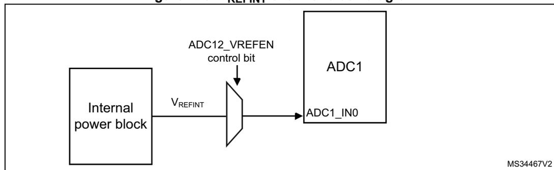
Note: The VREFEN bit into ADCx\_CCR register must be set to enable the conversion of internal channels ADC1\_IN0 ( $V_{REFINT}$ ).
