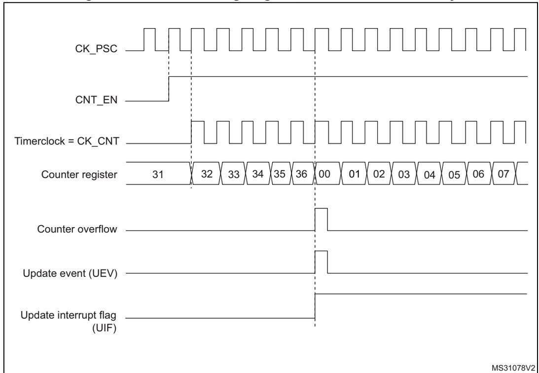
**Figure 274. Counter timing diagram, internal clock divided by 2**
