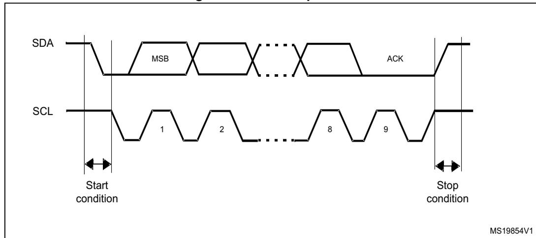
Acknowledge can be enabled or disabled by software. The I2C interface addresses can be selected by software.
