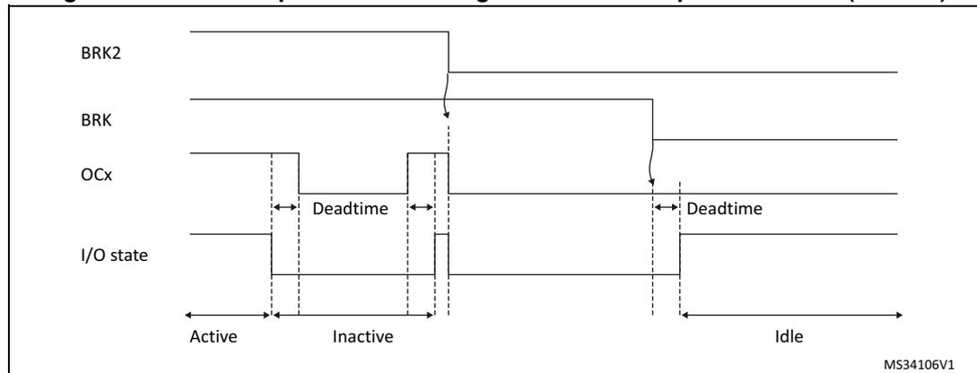
Figure 206. PWM output state following BRK assertion (OSSI=0)
