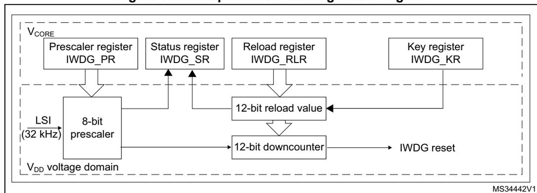
*Note:* The watchdog function is implemented in the  $V_{CORE}$  voltage domain that is still functional in Stop and Standby modes.
