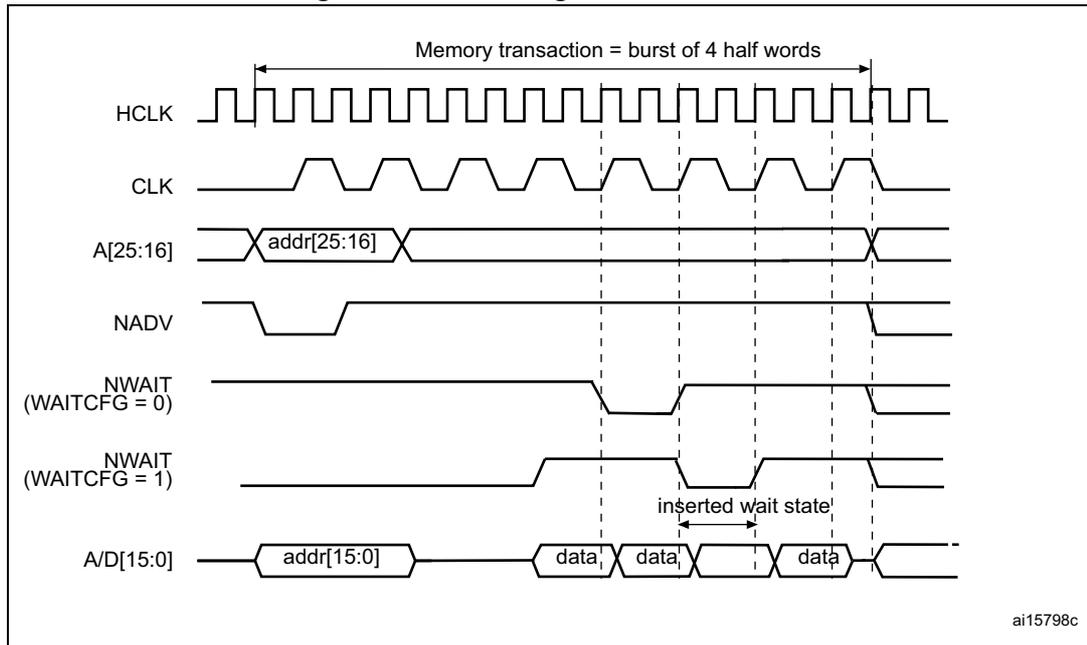
Figure 47. Synchronous multiplexed read mode waveforms - NOR, PSRAM (CRAM)
