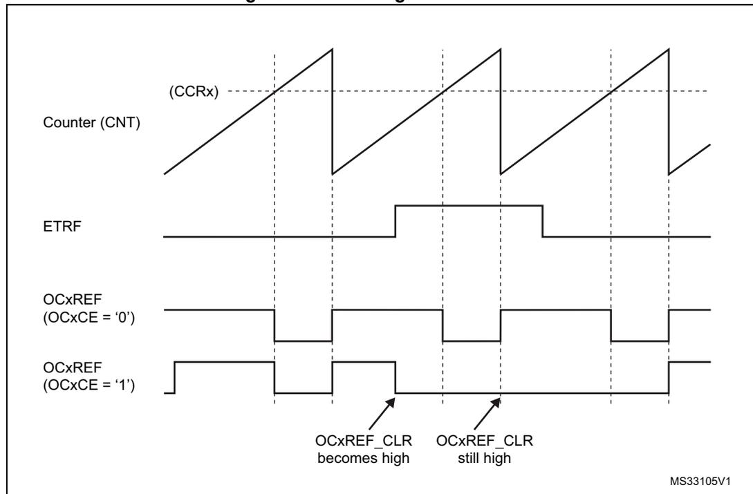
Note: In case of a PWM with a 100% duty cycle (if  $CCR_x > ARR$ ), then OCxREF is enabled again at the next counter overflow.
