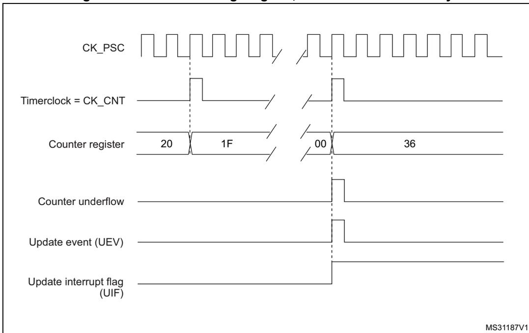
**Figure 233. Counter timing diagram, Update event when repetition counter is not used**
