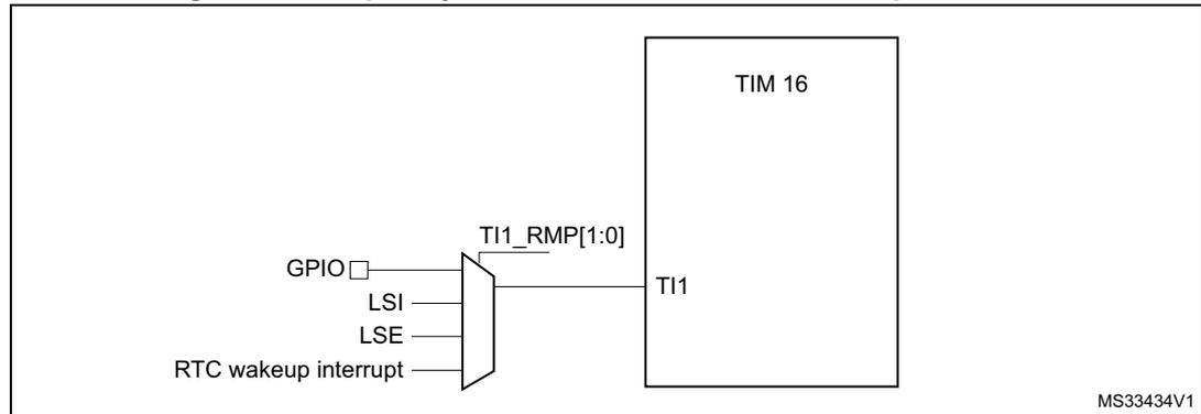
The input capture channel of the Timer 16 can be a GPIO line or an internal clock of the MCU. This selection is performed through the TI1\_RMP[1:0] bits in the TIM16\_OR register. The possibilities are the following ones:
