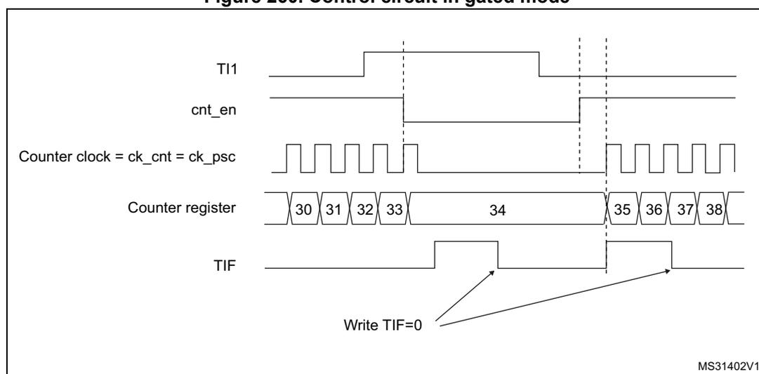
1. The configuration "CCxP=CCxNP=1" (detection of both rising and falling edges) does not have any effect in gated mode because gated mode acts on a level and not on an edge.
