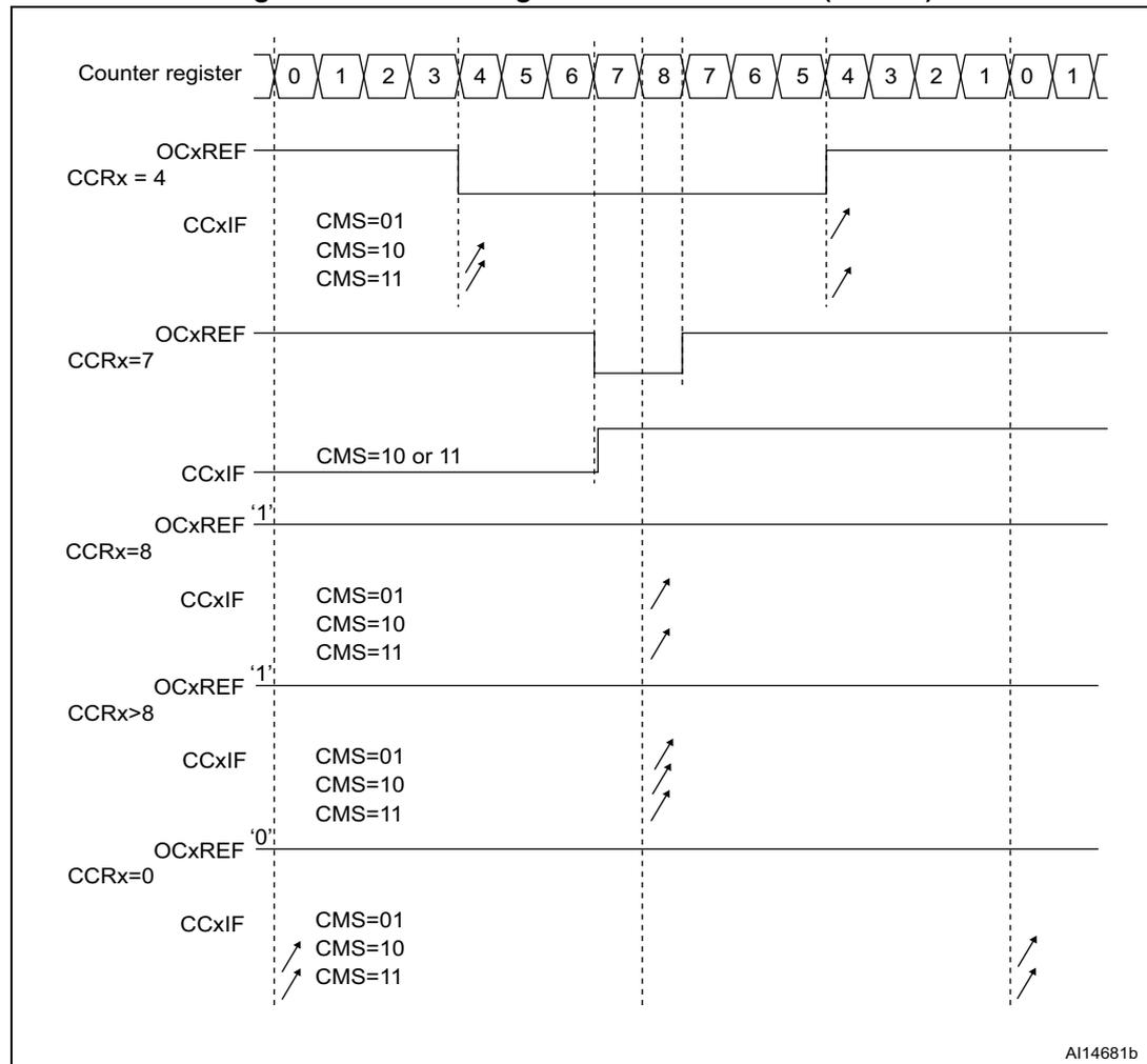
**Hints on using center-aligned mode**
