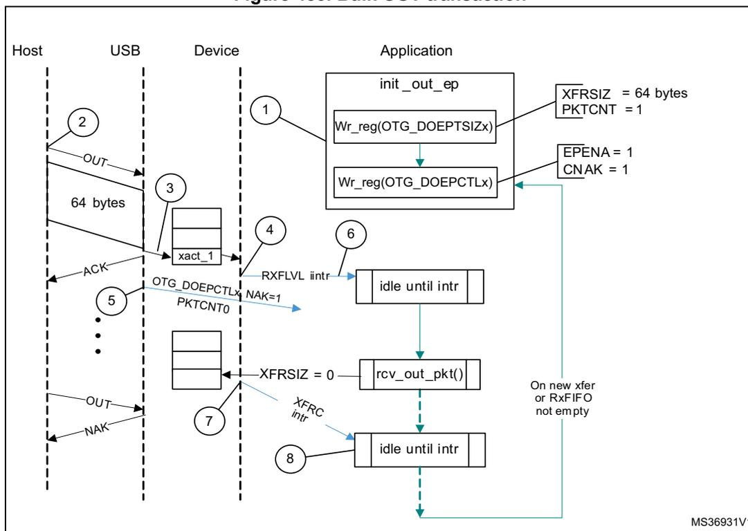
After a SetConfiguration/SetInterface command, the application initializes all OUT endpoints by setting  $\text{CNAK} = 1$  and  $\text{EPENA} = 1$  (in  $\text{OTG\_DOEPTCLx}$ ), and setting a suitable  $\text{XFRSIZ}$  and  $\text{PKTCNT}$  in the  $\text{OTG\_DOEPTSIZx}$  register.
