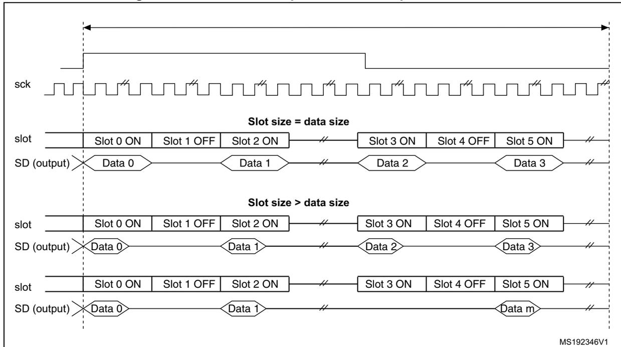
If the TRIS bit in the SAI\_xCR2 register is cleared, all the High impedance states on the SD output line on [Figure 419](#) and [Figure 420](#) are replaced by a drive with a value of 0.
