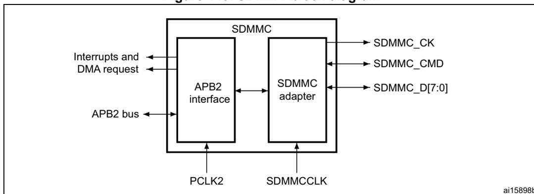
By default SDMMC\_D0 is used for data transfer. After initialization, the host can change the databus width.
