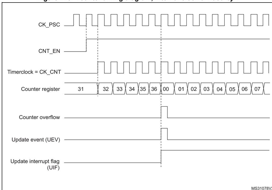
**Figure 224. Counter timing diagram, internal clock divided by 2**
