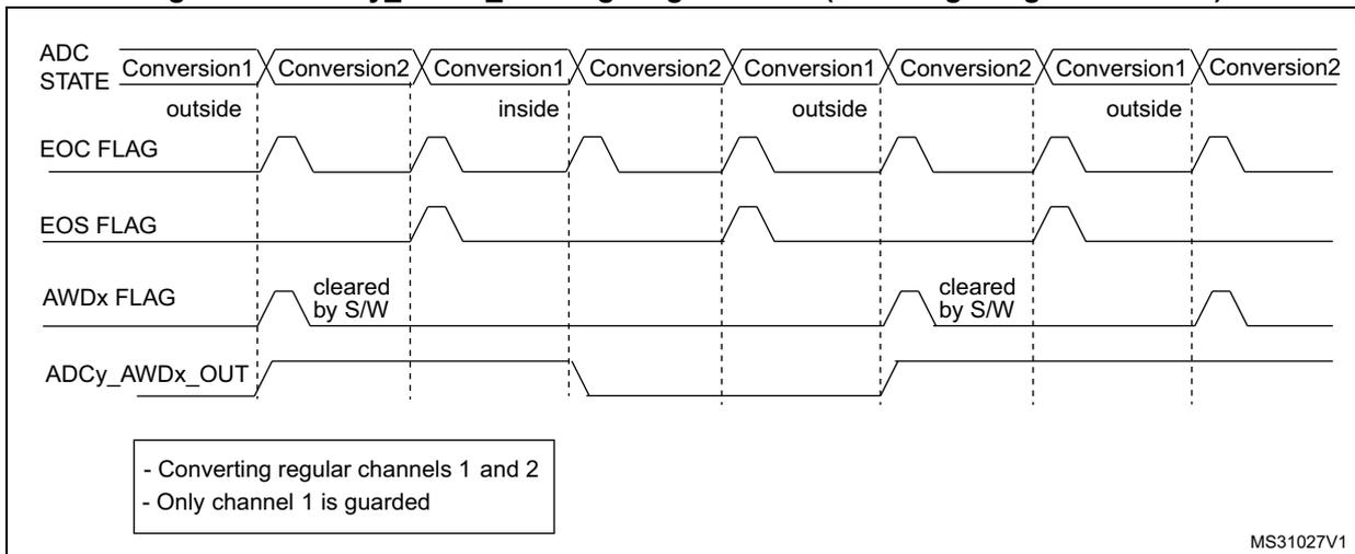
Figure 102. ADCy\_AWDx\_OUT signal generation (on all injected channels)
