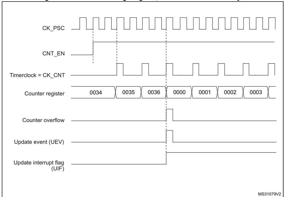
Figure 275. Counter timing diagram, internal clock divided by 4
