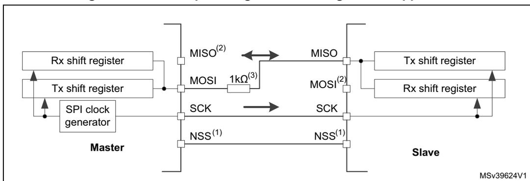
1. The NSS pins can be used to provide a hardware control flow between master and slave. Optionally, the pins can be left unused by the peripheral. Then the flow has to be handled internally for both master and slave. For more details see [Section 36.4.5: Slave select \(NSS\) pin management](#).
