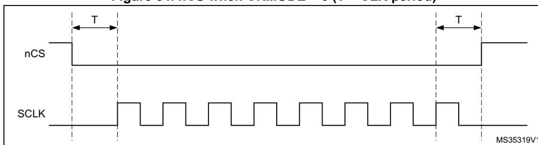
When CKMODE=1 (“mode3”, where CLK goes high when no operation is in progress) and DDRM=0 (SDR mode), nCS still falls one CLK cycle before an operation first rising CLK edge, and nCS rises one CLK cycle after the operation final rising CLK edge, as shown in [Figure 55](#).
