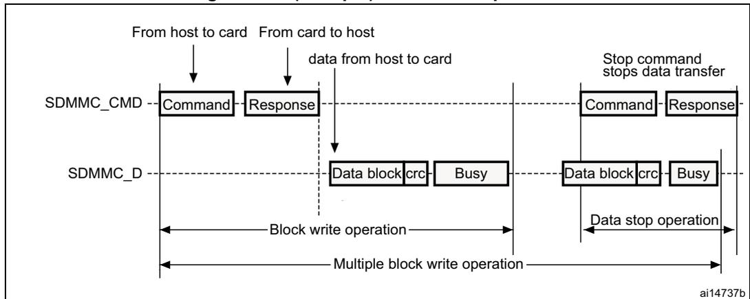
Note: The SDMMC will not send any data as long as the Busy signal is asserted (SDMMC\_D0 pulled low).
