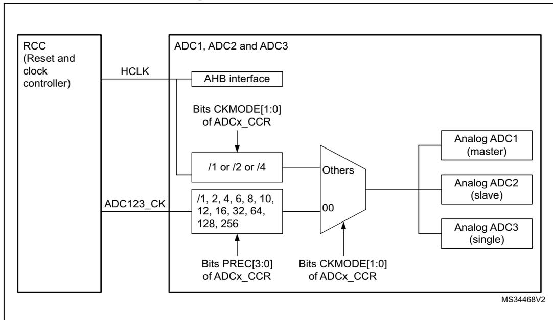
**Clock ratio constraint between ADC clock and AHB clock**
