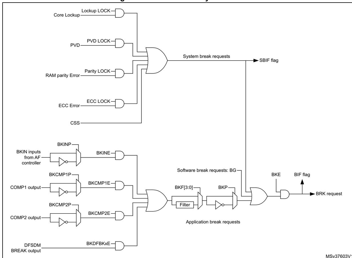
**Note:** *An asynchronous (clockless) operation is only guaranteed when the programmable filter is disabled. If it is enabled, a fail safe clock mode (for example by using the internal PLL and/or the CSS) must be used to guarantee that break events are handled.*
