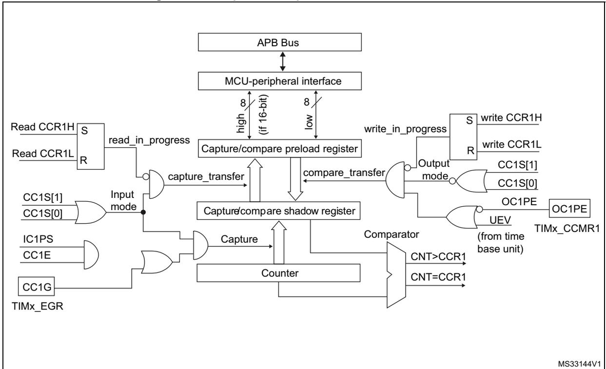
Figure 247. Output stage of capture/compare channel (channel 1)
