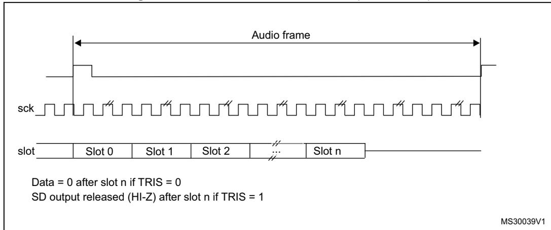
The FS signal is not used when the audio block in transmitter mode is configured to get the SPDIF output on the SD line. The corresponding FS I/O will be released and left free for other purposes.
