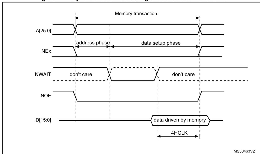
1. NWAIT polarity depends on WAITPOL bit setting in FMC\_BCRx register.
