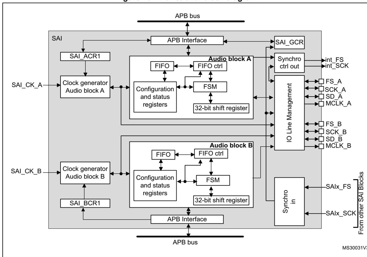
The SAI is mainly composed of two audio sub-blocks with their own clock generator. Each audio block integrates a 32-bit shift register controlled by their own functional state machine. Data are stored or read from the dedicated FIFO. FIFO may be accessed by the CPU, or by DMA in order to leave the CPU free during the communication. Each audio block is independent. They can be synchronous with each other.
