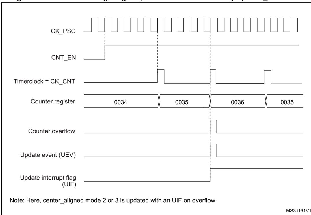
Note: Here, center\_aligned mode 2 or 3 is updated with an UIF on overflow
