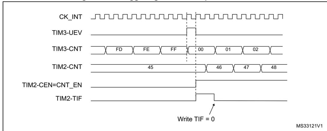
As in the previous example, you can initialize both counters before starting counting. [Figure 267](#) shows the behavior with the same configuration as in [Figure 266](#) but in trigger mode instead of gated mode (SMS=110 in the TIM2\_SMCR register).
