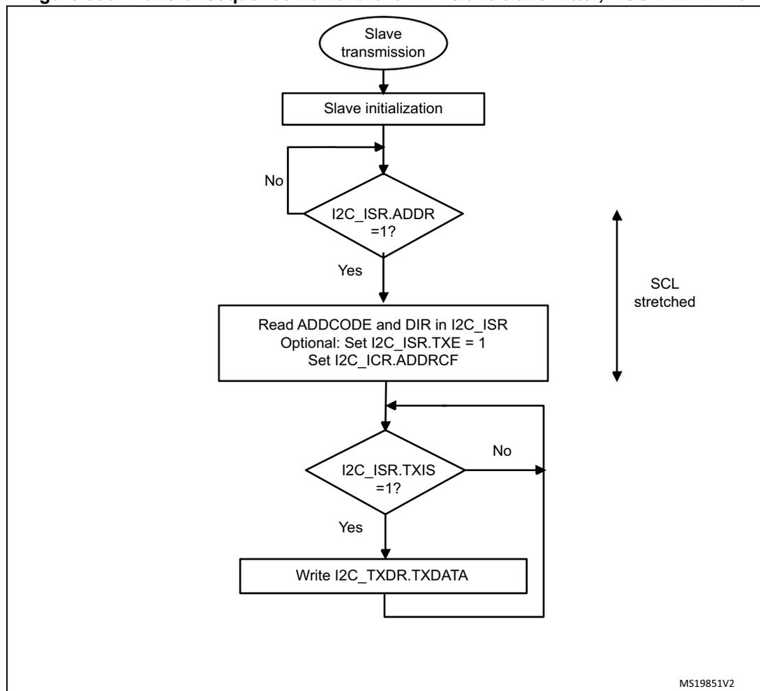
Figure 331. Transfer sequence flowchart for I2C slave transmitter, NOSTRETCH=1
