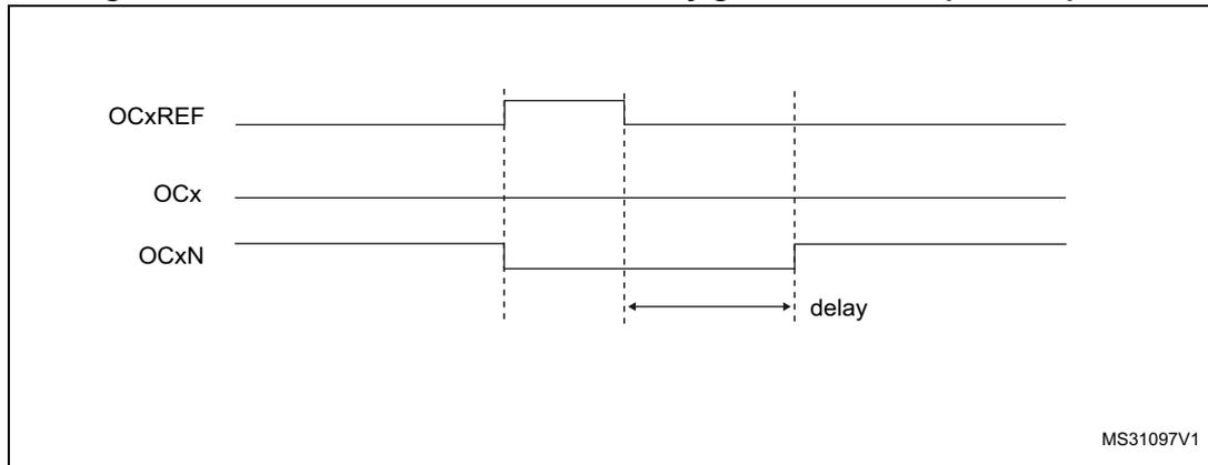
The dead-time delay is the same for each of the channels and is programmable with the DTG bits in the TIMx\_BDTR register. Refer to [Section 24.4.18: TIM1/TIM8 break and dead-time register \(TIMx\\_BDTR\) on page 761](#) for delay calculation.
