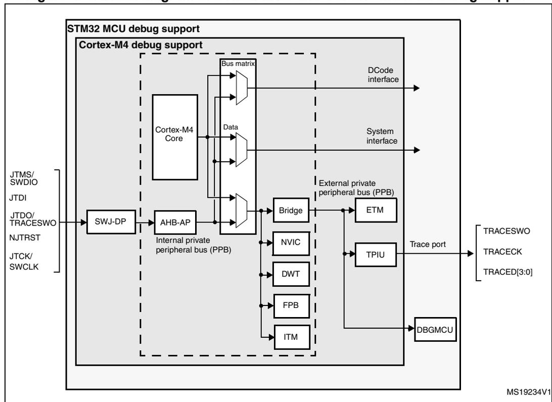
*Note:* The debug features embedded in the Cortex<sup>®</sup>-M4 core are a subset of the ARM<sup>®</sup> CoreSight Design Kit.
