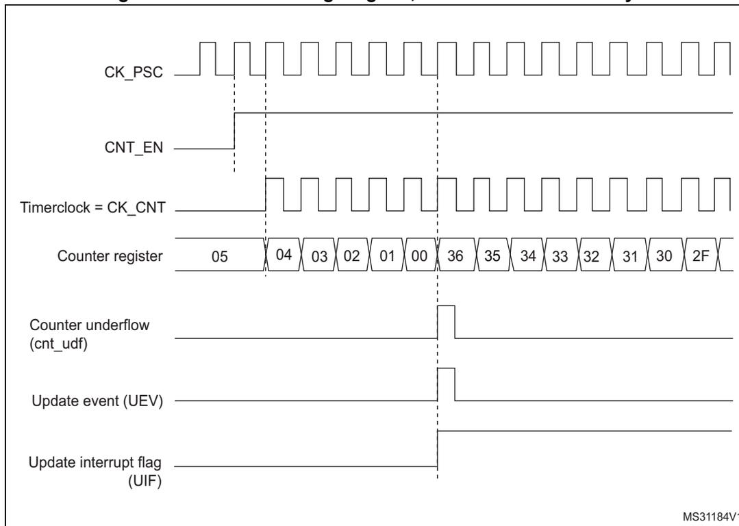
Figure 169. Counter timing diagram, internal clock divided by 2
