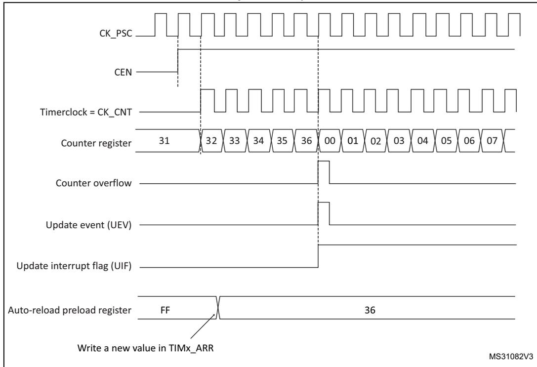
**Figure 167. Counter timing diagram, update event when ARPE=1 (TIMx\_ARR preloaded)**
