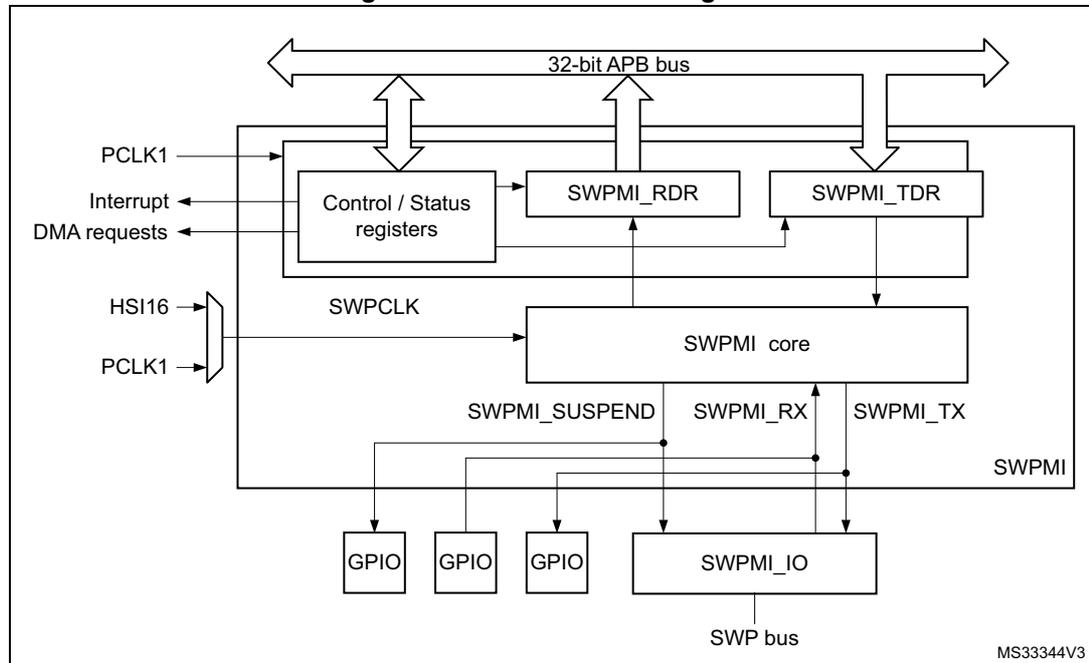
Refer to the bit SWPMI1SEL in [Section 6.4.28: Peripherals independent clock configuration register \(RCC\\_CCIPR\)](#) to select the SWPCLK (SWPMI core clock source).
