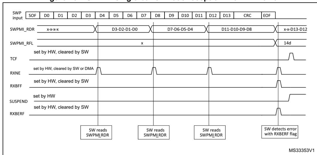
**Missing or corrupted stuffing bit during payload reception**
