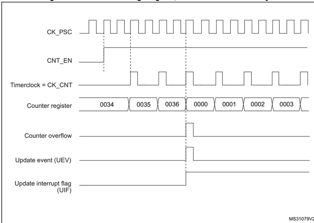
Figure 306. Counter timing diagram, internal clock divided by 4
