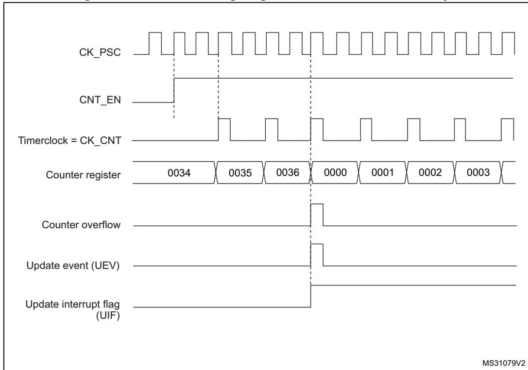
**Figure 225. Counter timing diagram, internal clock divided by 4**
