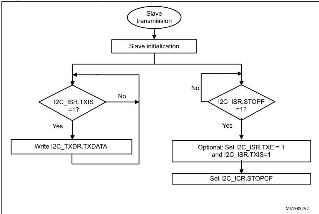
Figure 332. Transfer bus diagrams for I2C slave transmitter
