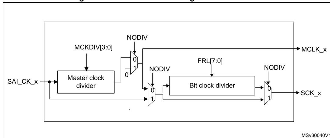
*Note:* If NODIV is set to 1, the MCLK\_x signal will be set at 0 level if this pin is configured as the SAI pin in GPIO peripherals.
