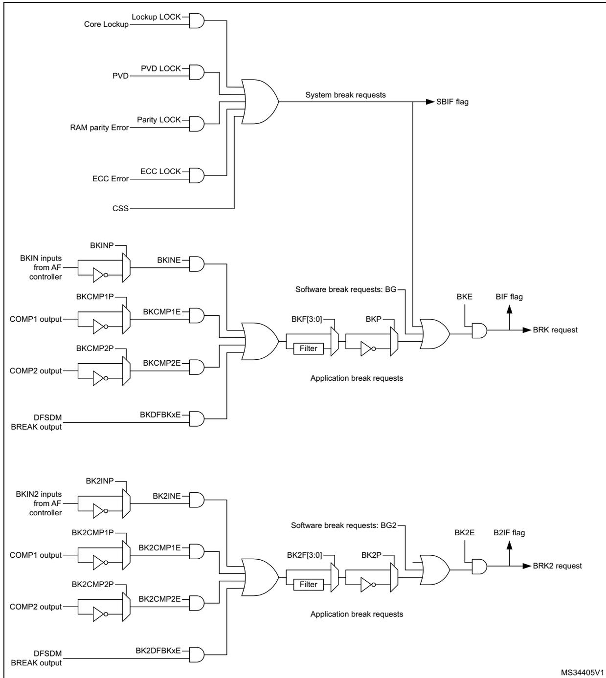
**Note:** An asynchronous (clockless) operation is only guaranteed when the programmable filter is disabled. If it is enabled, a fail safe clock mode (for example by using the internal PLL and/or the CSS) must be used to guarantee that break events are handled.
