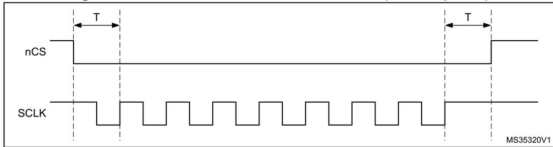
When CKMODE = 1 ("mode3") and DDRM = 1 (DDR mode), nCS falls one CLK cycle before an operation first rising CLK edge, and nCS rises one CLK cycle after the operation final active rising CLK edge, as shown in [Figure 56](#). Because DDR operations must finish with a falling edge, CLK is low when nCS rises, and CLK rises back up one half of a CLK cycle afterwards.
