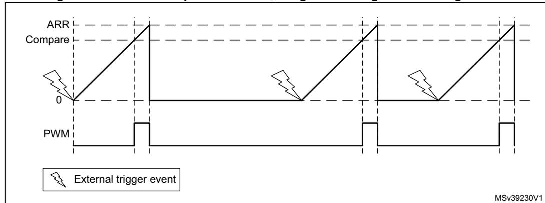
It should be noted that when the WAVE bit-field in the LPTIMx\_CFGR register is set, the Set-once mode is activated. In this case, the counter is only started once following the first trigger, and any subsequent trigger event is discarded as shown in [Figure 314](#).
