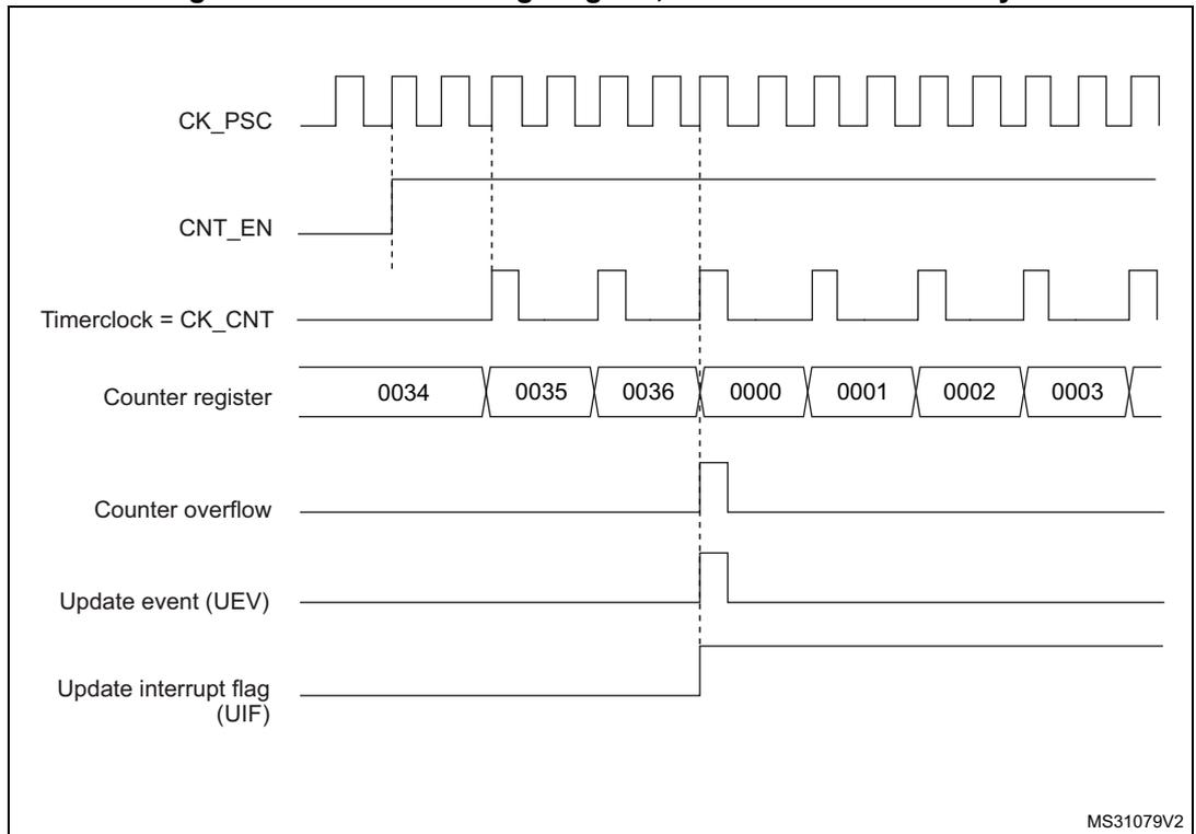
Figure 164. Counter timing diagram, internal clock divided by 4
