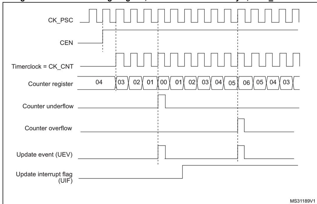
1. Here, center-aligned mode 1 is used (for more details refer to [Section 25.4.1: TIMx control register 1 \(TIMx\\_CR1\) on page 828](#)).
