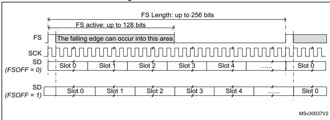
In AC'97 mode or in SPDIF mode (bit PRTCFCFG[1:0] = 10 or PRTCFCFG[1:0] = 01 in the SAI\_xCR1 register), the frame synchronization shape is forced to match the AC'97 protocol. The SAI\_xFRCR register value is ignored.
