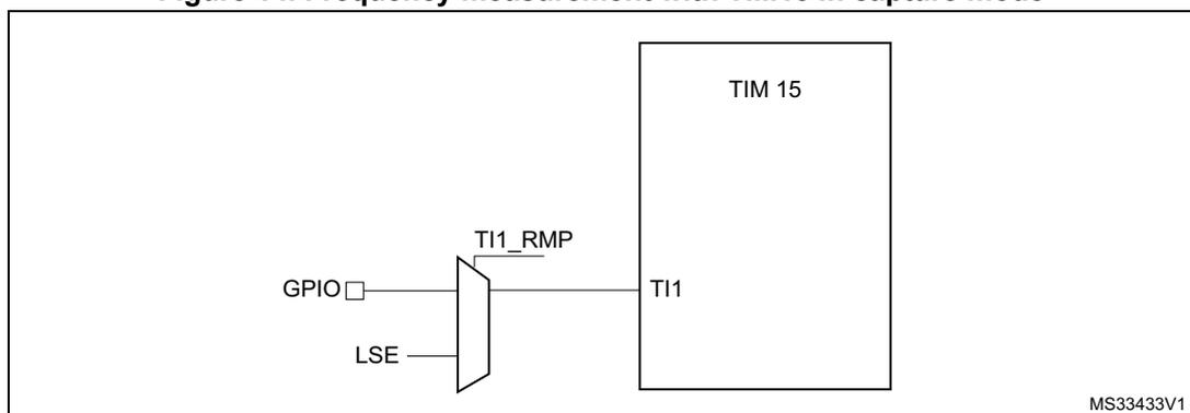
The input capture channel of the Timer 15 can be a GPIO line or an internal clock of the MCU. This selection is performed through the TI1\_RMP bit in the TIM15\_OR register. The possibilities are the following ones:
