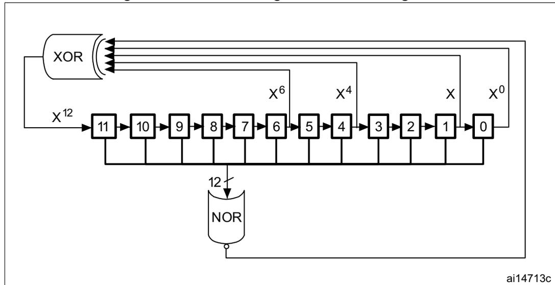
The LFSR value, that may be masked partially or totally by means of the MAMPx[3:0] bits in the DAC\_CR register, is added up to the DAC\_DHRx contents without overflow and this value is then transferred into the DAC\_DORx register.
