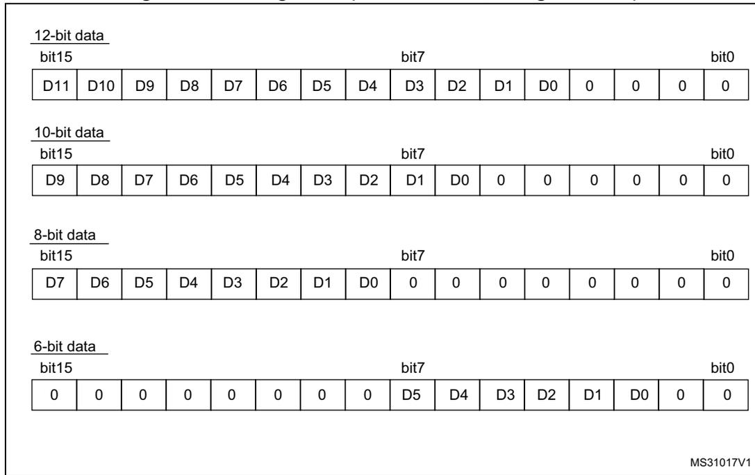
**Figure 91. Left alignment (offset enabled, signed value)**
