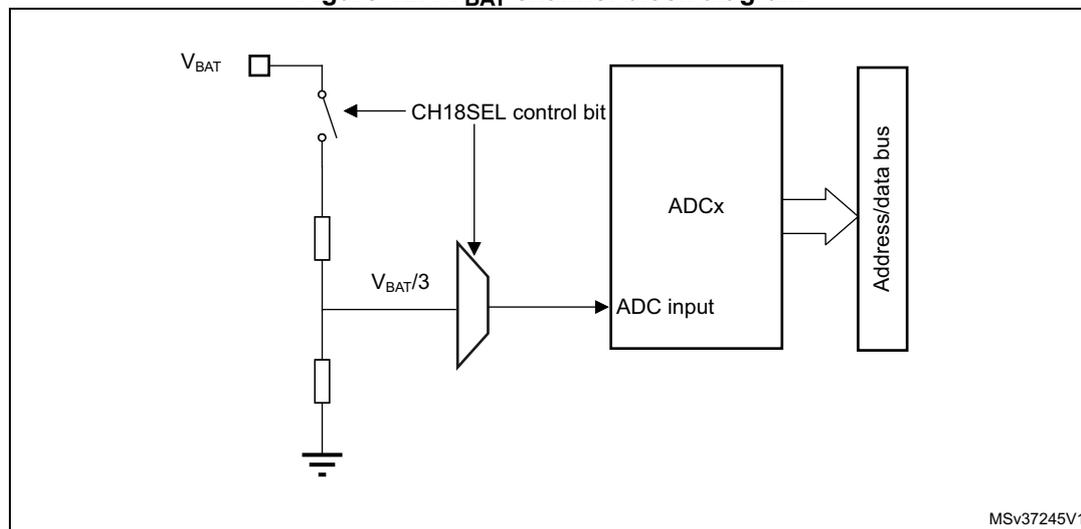
*Note:* The CH18\_SEL bit must be set to enable the conversion of internal channels ADC1\_IN18 and ADC3\_IN18 ( $V_{BAT}/3$ ).
