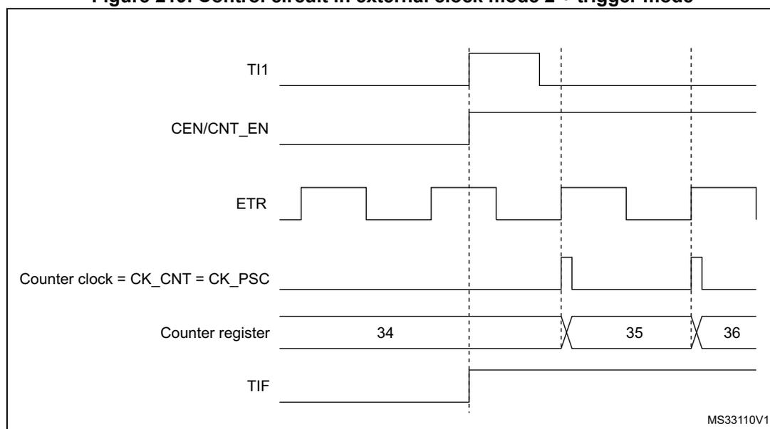
*Note:* The clock of the slave timer must be enabled prior to receive events from the master timer, and must not be changed on-the-fly while triggers are received from the master timer.
