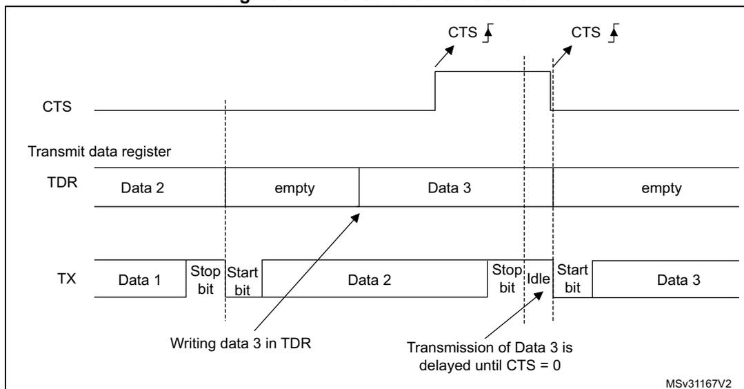
**Note:** For correct behavior, CTS must be asserted at least 3 USART clock source periods before the end of the current character. In addition it should be noted that the CTSCF flag may not be set for pulses shorter than 2 x PCLK periods.
