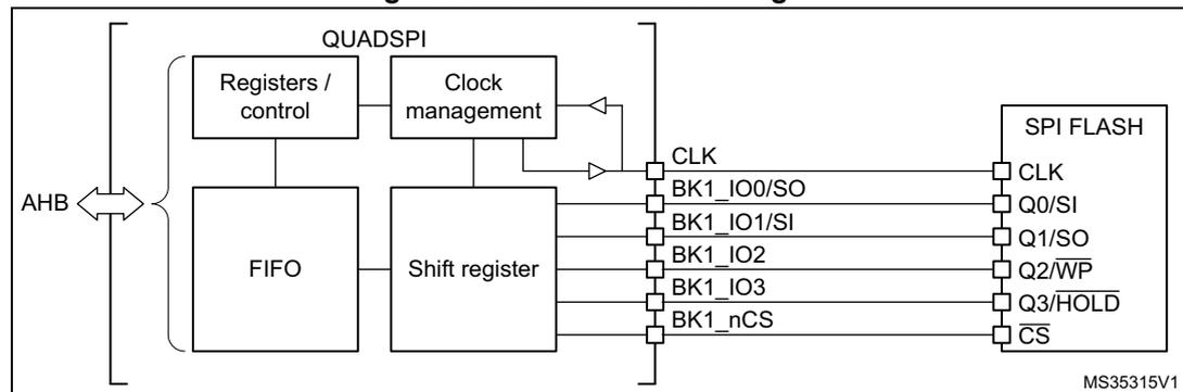
The QUADSPI uses 6 signals to interface with a Flash memory:
