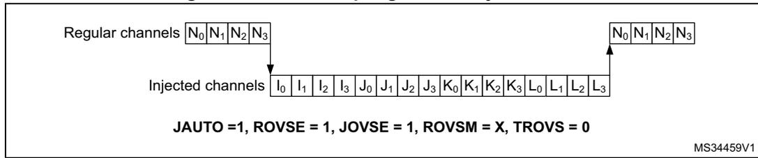
It is possible to have also the triggered mode enabled, using the TROVS bit. In this case, the ADC must be configured as following: JAUTO = 1, DISCEN = 0, JDISCEN = 0, ROVSE = 1, JOVSE = 1 and TROVSE = 1.
