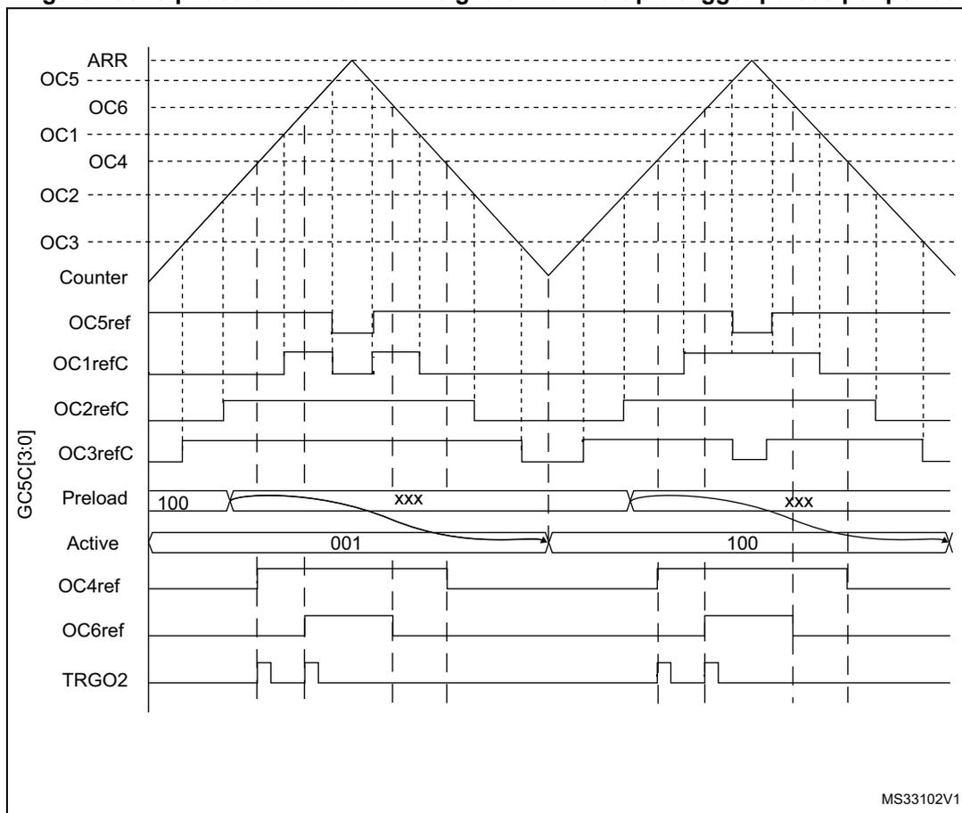
The TRGO2 waveform shows how the ADC can be synchronized on given 3-phase PWM signals. Please refer to [Section 24.3.27: ADC synchronization](#) for more details.
