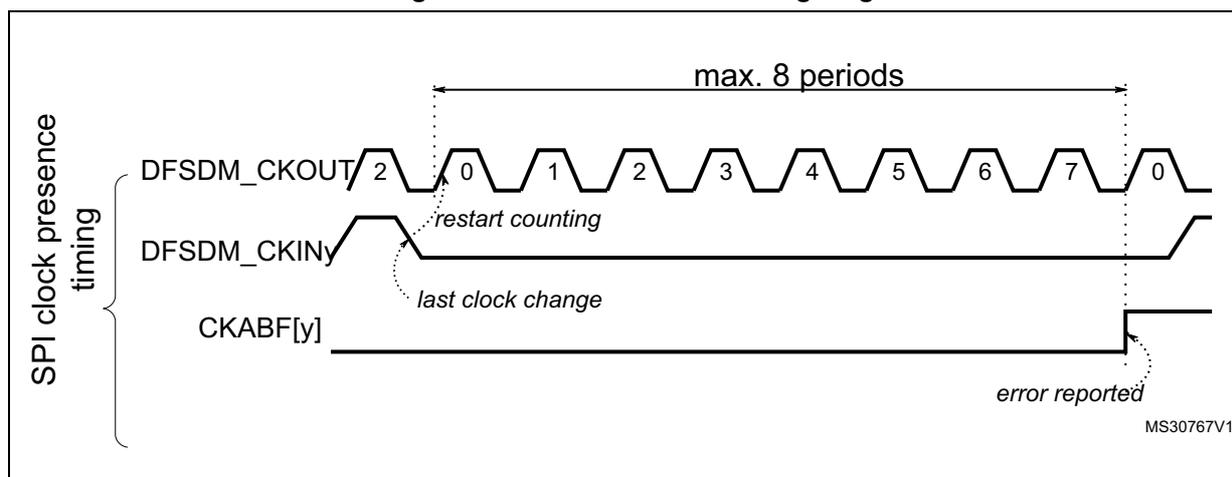
If Manchester data format is used, then the clock absence means that the clock recovery is unable to perform from Manchester coded signal. For a correct clock recovery, it is first necessary to receive data with 1 to 0 or 0 to 1 transition (see [Figure 150](#) for Manchester synchronization).
