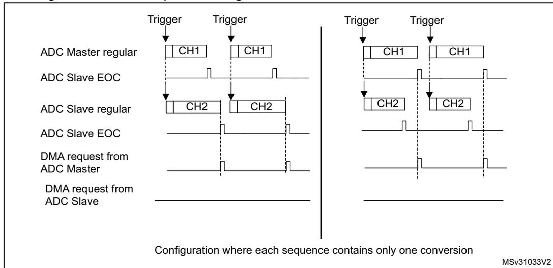
**Figure 125. DMA requests in interleaved mode when MDMA=0b10**
