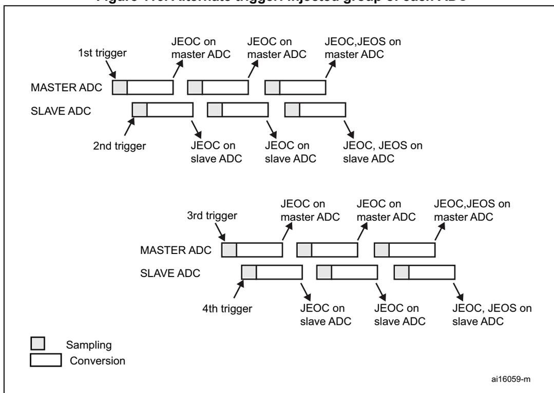
**Note:** Regular conversions can be enabled on one or all ADCs. In this case the regular conversions are independent of each other. A regular conversion is interrupted when the ADC has to perform an injected conversion. It is resumed when the injected conversion is finished.
