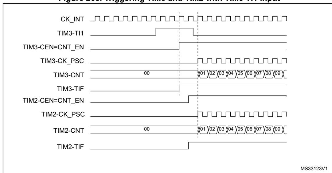
*Note: The clock of the slave timer must be enabled prior to receive events from the master timer, and must not be changed on-the-fly while triggers are received from the master timer.*
