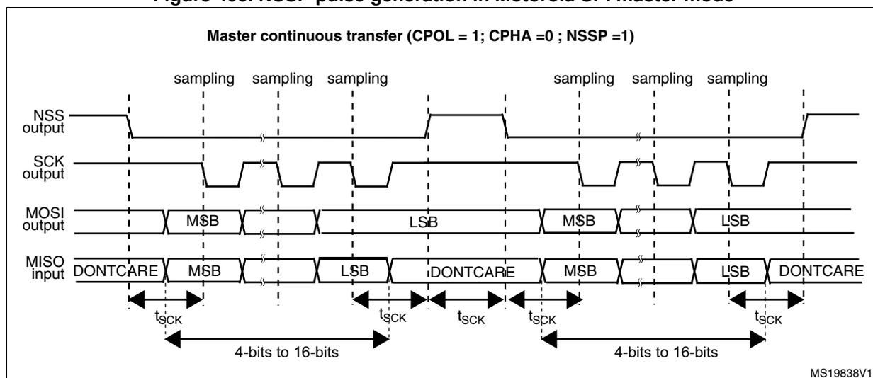
Note: Similar behavior is encountered when CPOL = 0. In this case the sampling edge is the rising edge of SCK, and NSS assertion and deassertion refer to this sampling edge.
