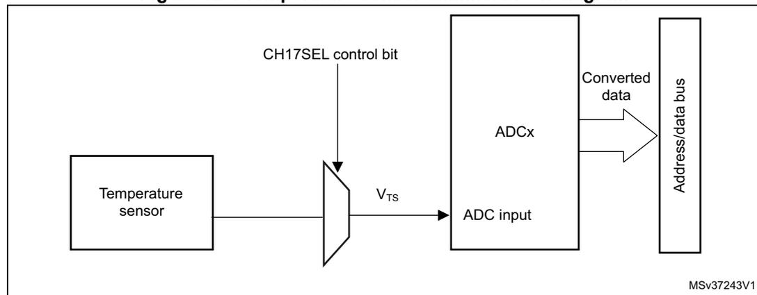
*Note:* The CH17SEL bit must be set to enable the conversion of the temperature sensor voltage  $V_{TS}$ .
