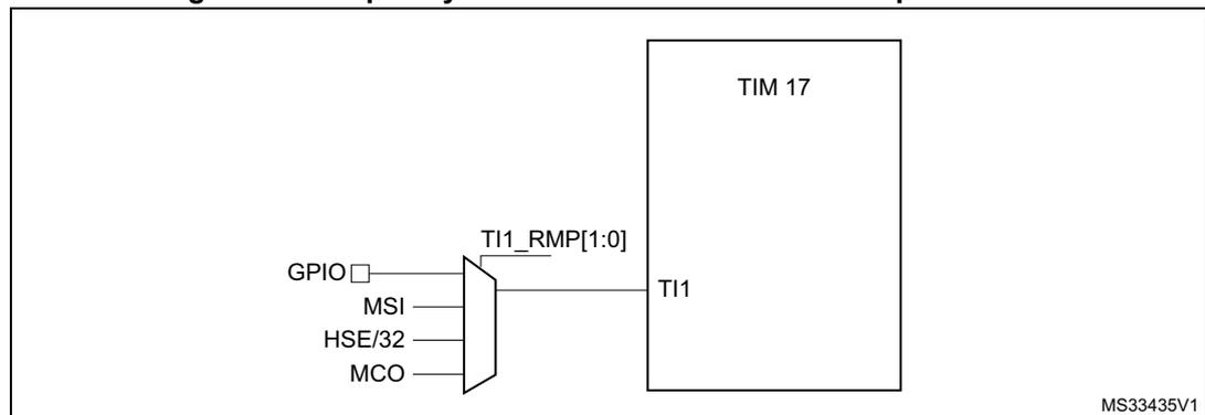
The input capture channel of the Timer 17 can be a GPIO line or an internal clock of the MCU. This selection is performed through the TI1\_RMP[1:0] bits in the TIM17\_OR register. The possibilities are the following ones:
