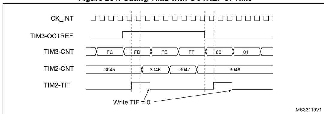
In the example in [Figure 264](#), the TIM2 counter and prescaler are not initialized before being started. So they start counting from their current value. It is possible to start from a given value by resetting both timers before starting TIM3. You can then write any value you want
