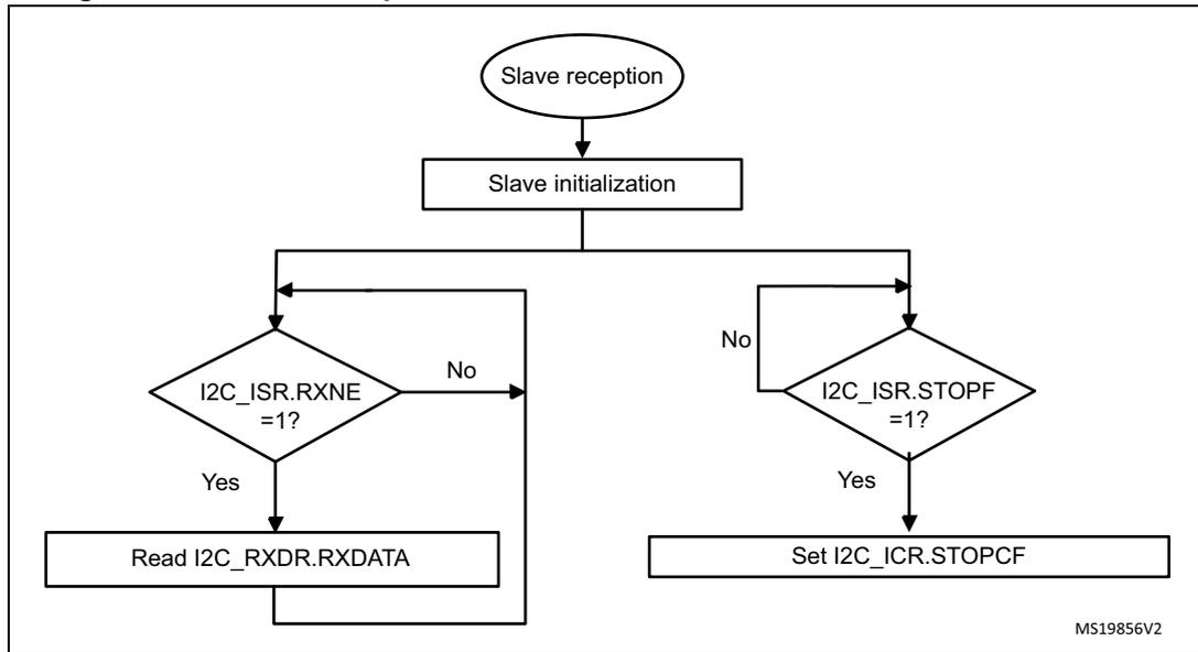
Figure 335. Transfer bus diagrams for I2C slave receiver
