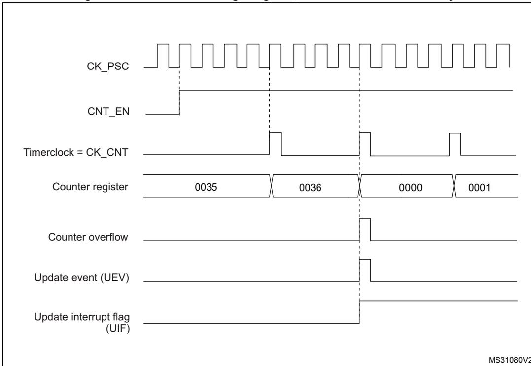
Figure 307. Counter timing diagram, internal clock divided by N
