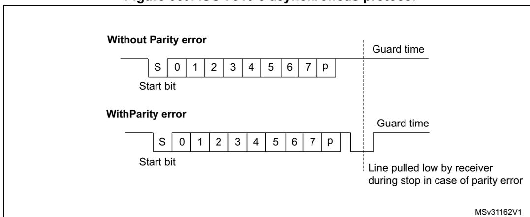
When connected to a smartcard, the TX output of the USART drives a bidirectional line that is also driven by the smartcard. The TX pin must be configured as open drain.
