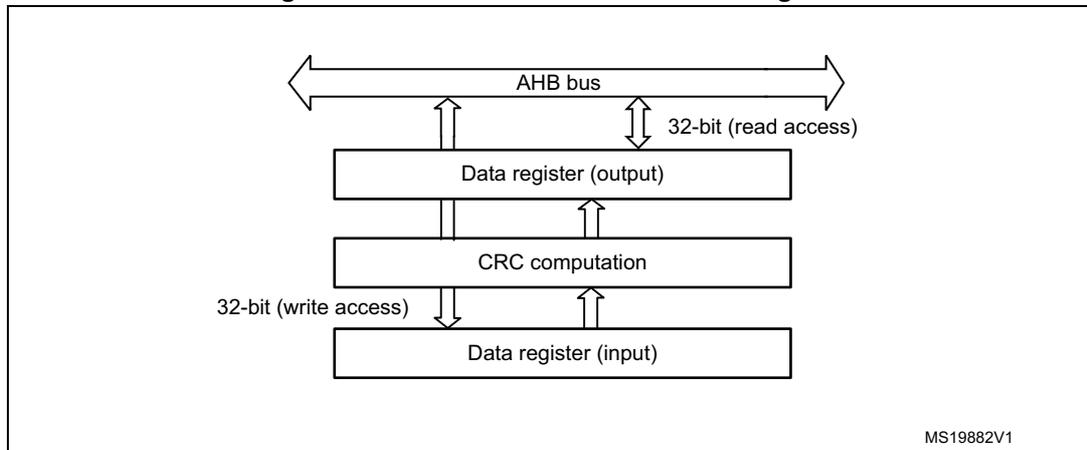
The CRC calculation unit has a single 32-bit read/write data register (CRC\_DR). It is used to input new data (write access), and holds the result of the previous CRC calculation (read access).
