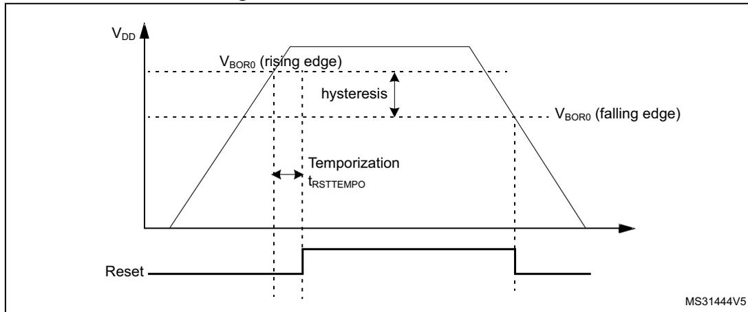
1. The reset temporization  $t_{RSTTEMPO}$  is present only for the BOR lowest threshold ( $V_{BOR0}$ ).
