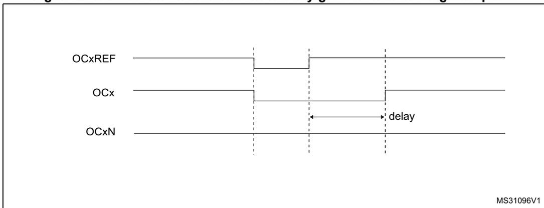
**Figure 202. Dead-time waveforms with delay greater than the positive pulse**
