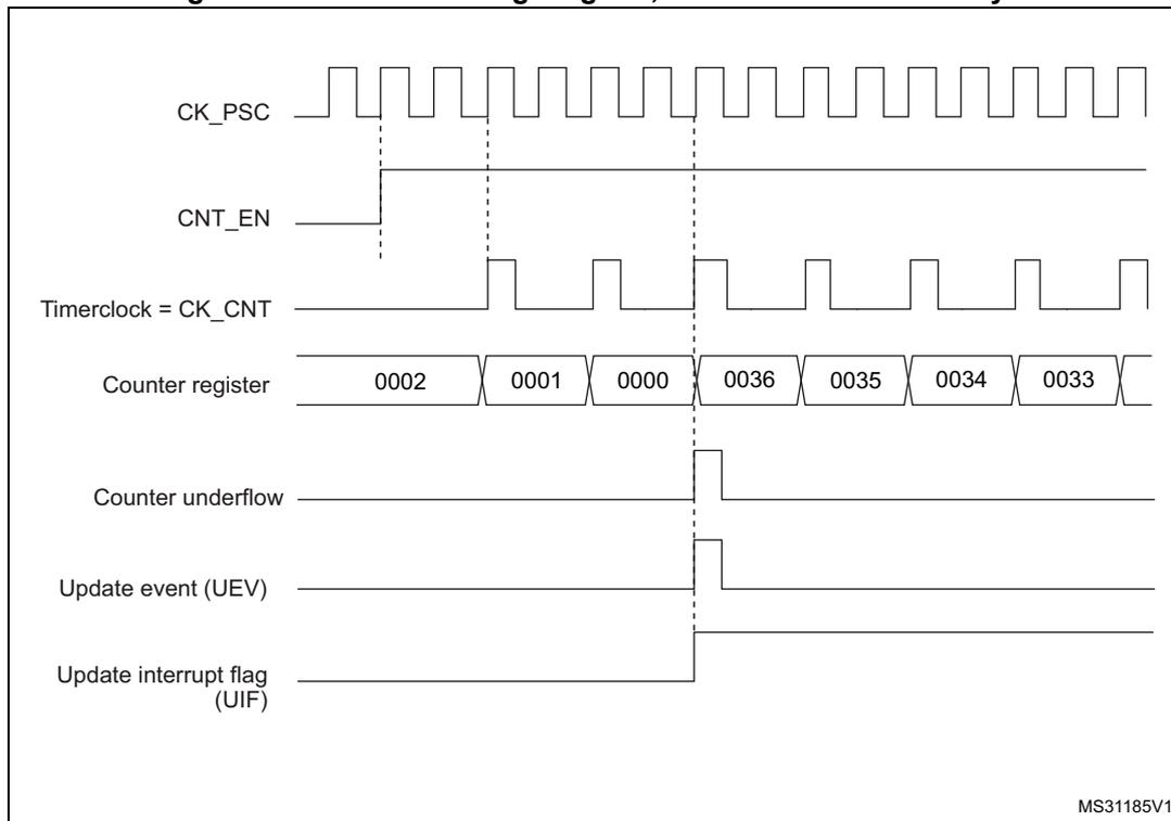
Figure 170. Counter timing diagram, internal clock divided by 4
