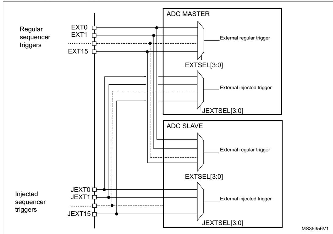
[Table 88](#) to [Table 89](#) give all the possible external triggers of the three ADCs for regular and injected conversion.
