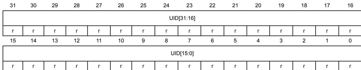
Bits 31:0 **UID[31:0]**: X and Y coordinates on the wafer
