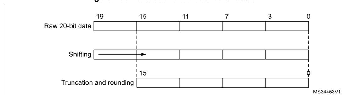
The [Figure 104](#) gives a numerical example of the processing, from a raw 20-bit accumulated data to the final 16-bit result.
