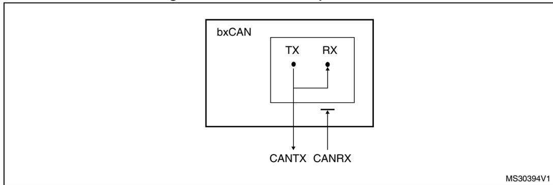
This mode is provided for self-test functions. To be independent of external events, the CAN Core ignores acknowledge errors (no dominant bit sampled in the acknowledge slot of a data / remote frame) in Loop Back Mode. In this mode, the bxCAN performs an internal feedback from its Tx output to its Rx input. The actual value of the CANRX input pin is disregarded by the bxCAN. The transmitted messages can be monitored on the CANTX pin.
