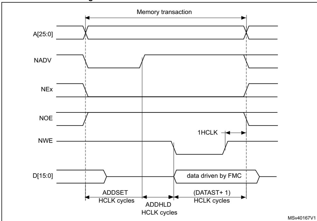
The differences with Mode1 are the toggling of NOE that goes on toggling after NADV changes and the independent read and write timings.
