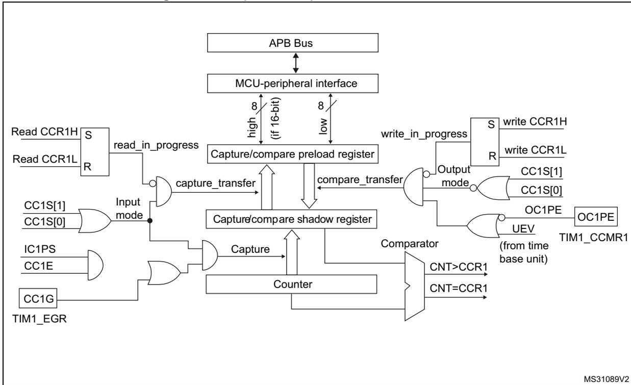
Figure 285. Output stage of capture/compare channel (channel 1)
