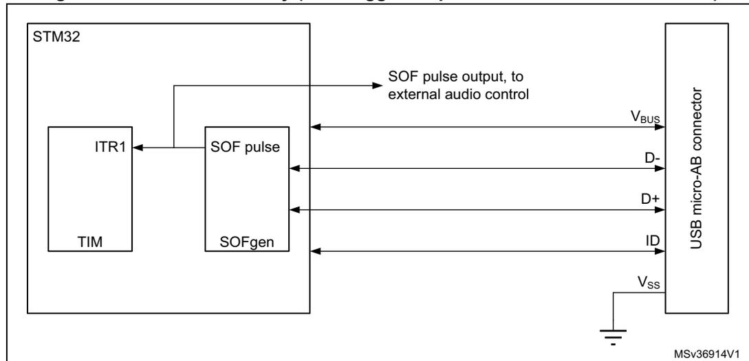
The OTG\_FS core provides means to monitor, track and configure SOF framing in the host and peripheral, as well as an SOF pulse output connectivity feature.
