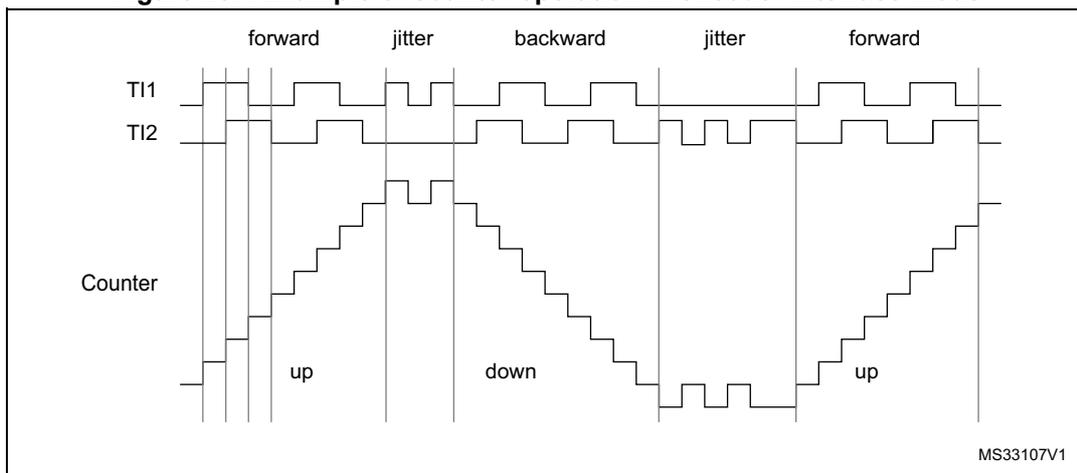
Figure 258 gives an example of counter behavior when TI1FP1 polarity is inverted (same configuration as above except CC1P=1).
