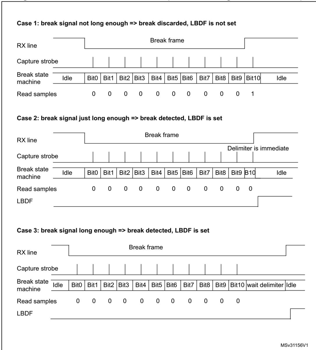
Figure 364. Break detection in LIN mode vs. Framing error detection
