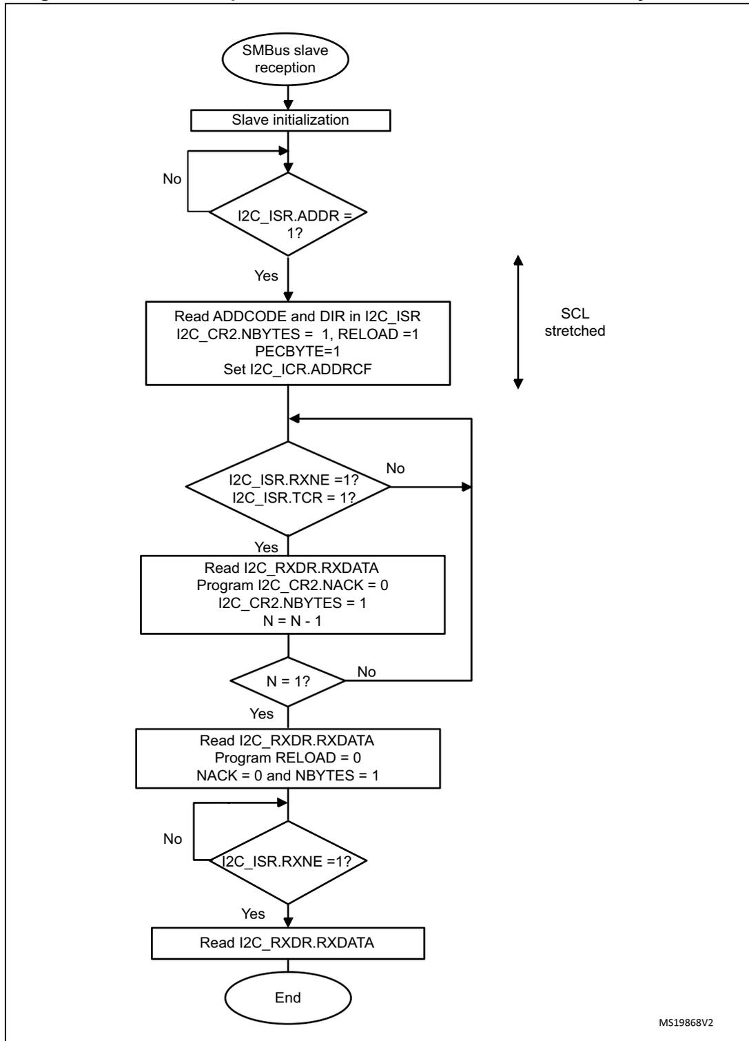
Figure 350. Bus transfer diagrams for SMBus slave receiver (SBC=1)
