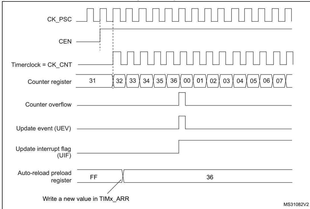
**Figure 278. Counter timing diagram, update event when ARPE=1 (TIMx\_ARR preloaded)**
