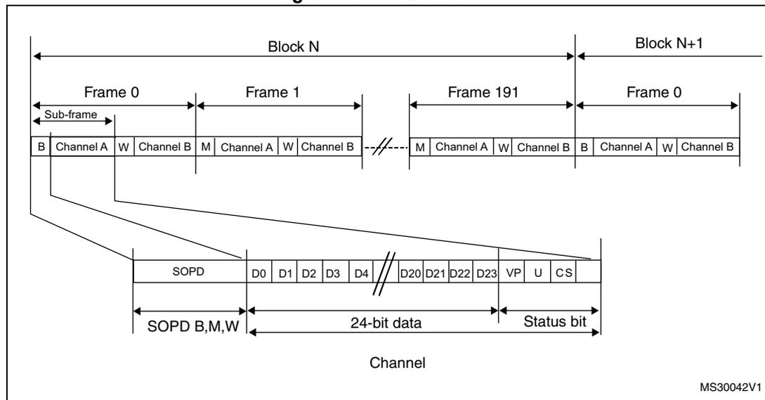
A SPDIF block contains 192 frames. Each frame is composed of two 32-bit sub-frames, generally one for the left channel and one for the right channel. Each sub-frame is composed of a SOPD pattern (4-bit) to specify if the sub-frame is the start of a block (and so is identifying a channel A) or if it is identifying a channel A somewhere in the block, or if it is referring to channel B (see [Table 199](#)). The next 28 bits of channel information are composed of 24 bits data + 4 status bits.
