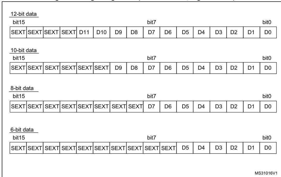
**Figure 90. Left alignment (offset disabled, unsigned value)**
