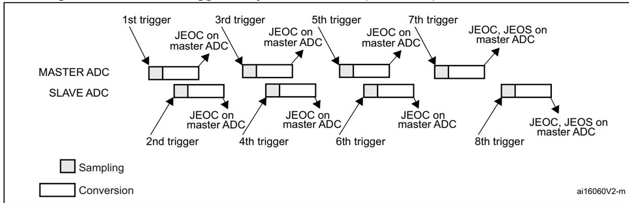
**Combined regular/injected simultaneous mode**
