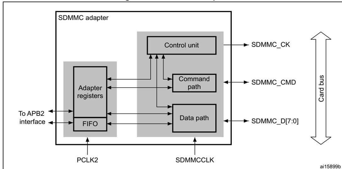
The SDMMC adapter is a multimedia/secure digital memory card bus master that provides an interface to a multimedia card stack or to a secure digital memory card. It consists of five subunits:
