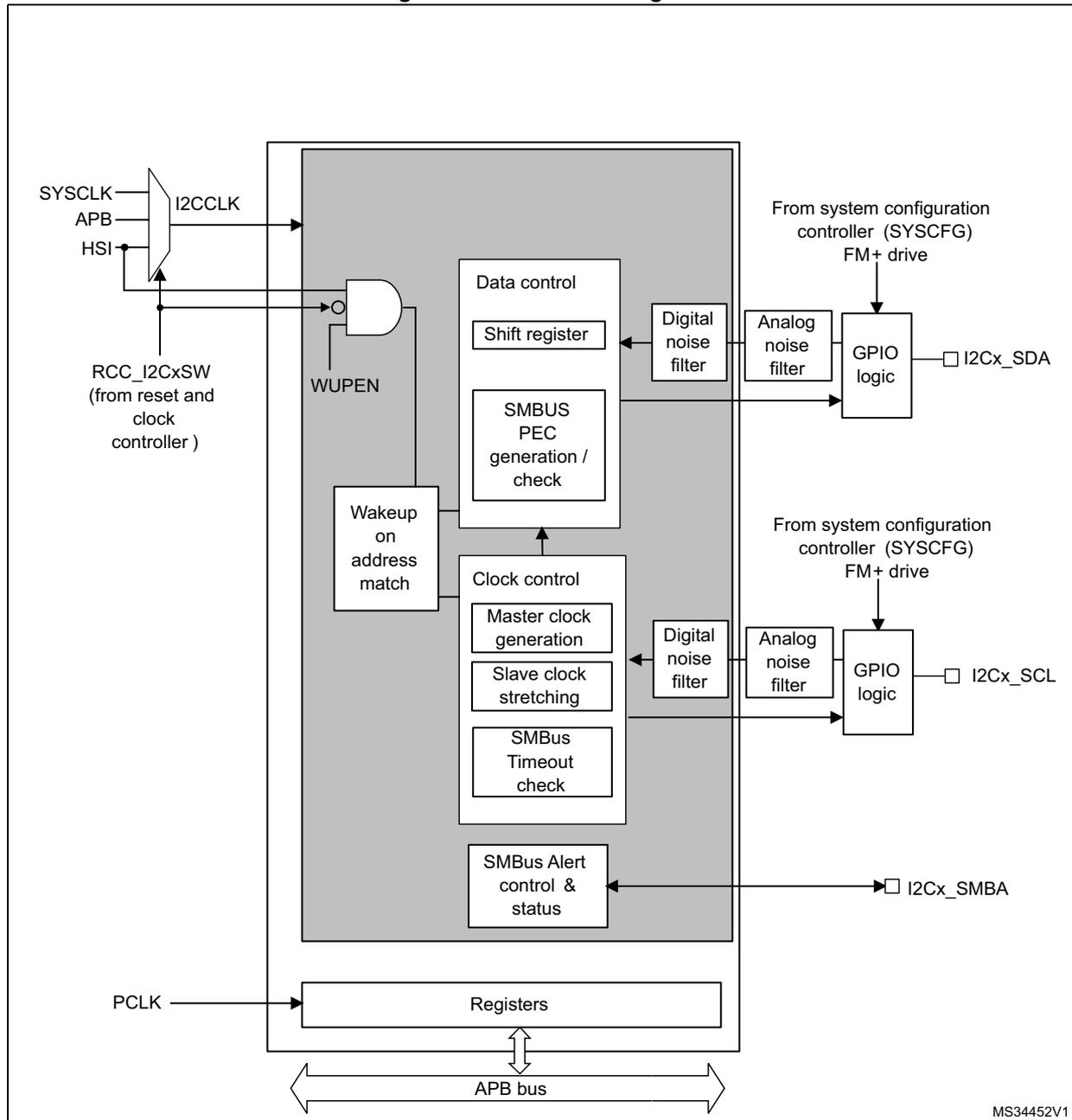
The I2C is clocked by an independent clock source which allows to the I2C to operate independently from the PCLK frequency.
