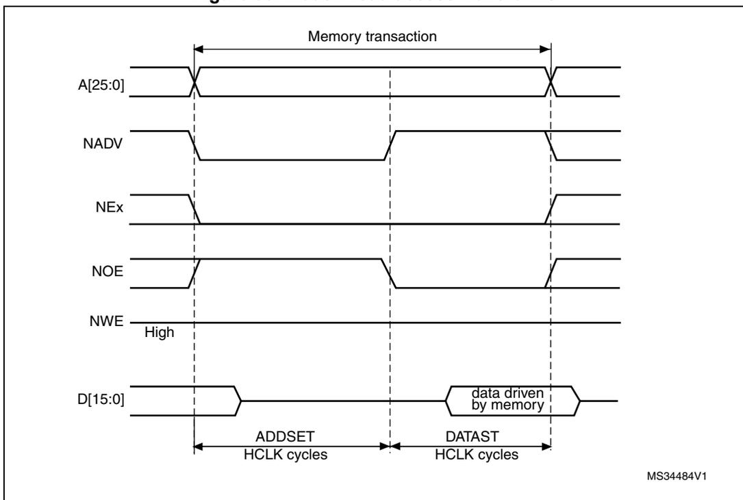
Figure 39. ModeC write access waveforms
