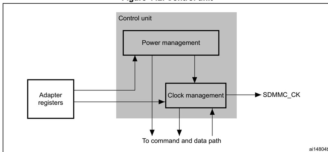
The control unit is illustrated in [Figure 442](#). It consists of a power management subunit and a clock management subunit.
