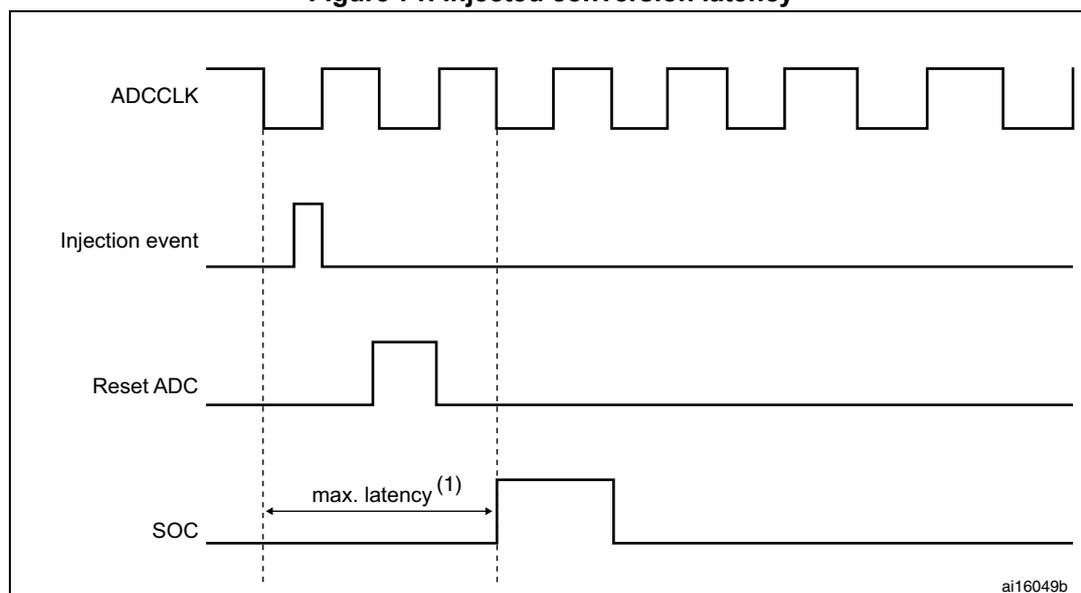
1. The maximum latency value can be found in the electrical characteristics of the STM32L4x5 datasheet.
