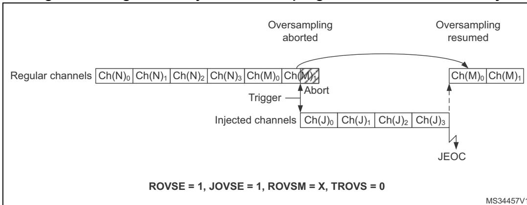
**Triggered regular oversampling with injected conversions**
