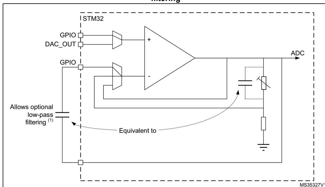
1. The gain depends on the cut-off frequency.
