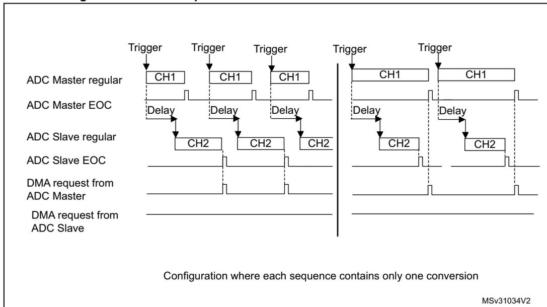
*Note:* When using MDMA mode, the user must take care to configure properly the duration of the master and slave conversions so that a DMA request is generated and served for reading both data (master + slave) before a new conversion is available.
