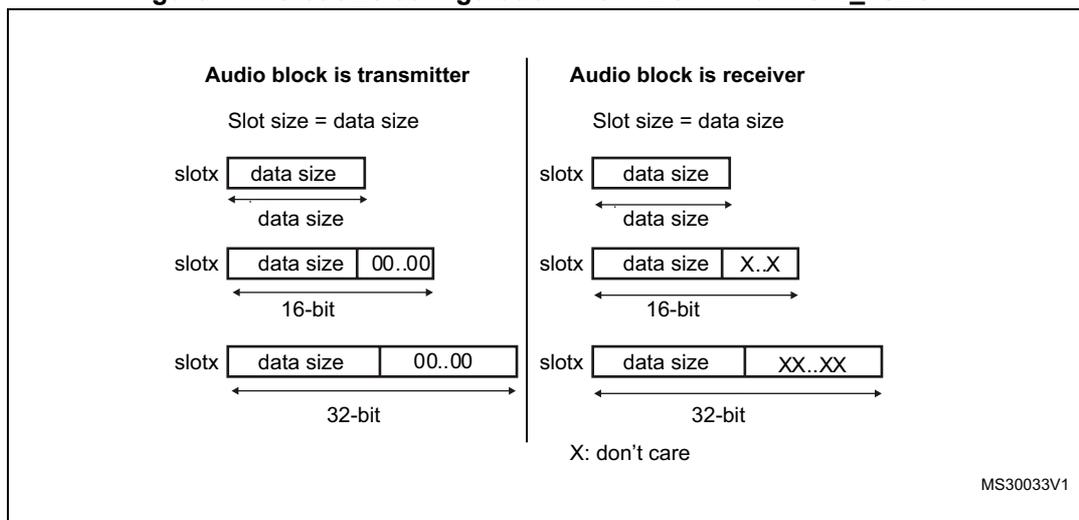
It is possible to choose the position of the first data bit to transfer within the slots. This offset is configured by FBOFF[4:0] bits in the SAI\_xSLOTR register. 0 values will be injected in transmitter mode from the beginning of the slot until this offset position is reached. In reception, the bit in the offset phase is ignored. This feature targets the LSB justified protocol (if the offset is equal to the slot size minus the data size).
