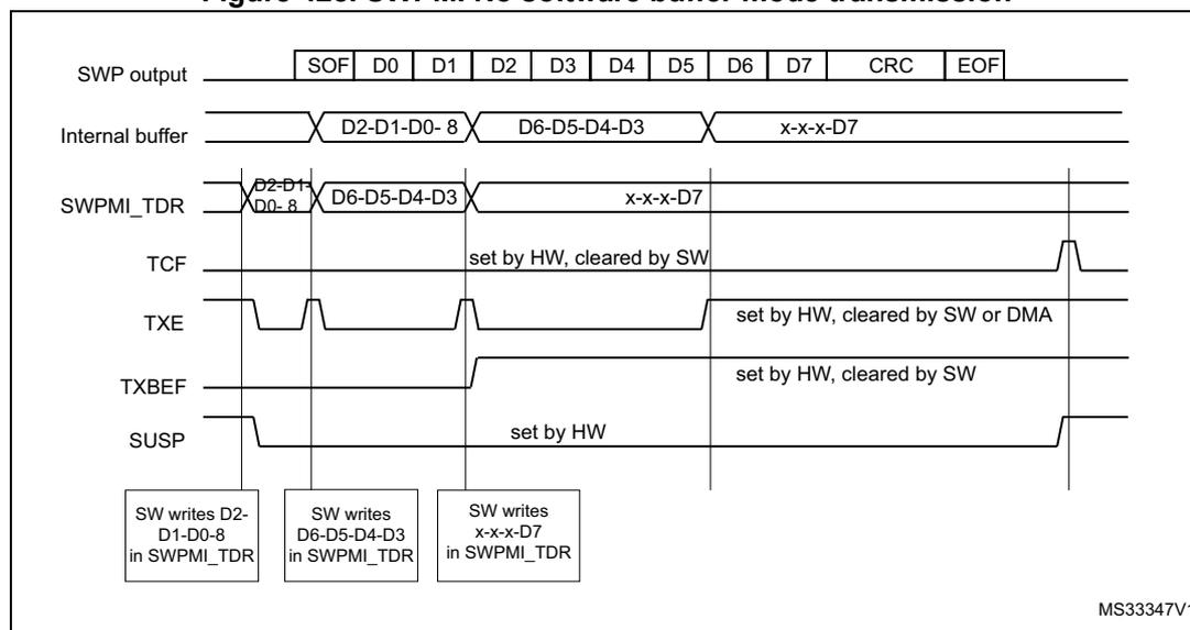
If another frame transmission is requested before the end of the EOF transmission, the TCF flag is not set and the frame will be consecutive to the previous one, with only one idle bit in between (refer to [Figure 429: SWPMI No software buffer mode transmission, consecutive frames](#)).
