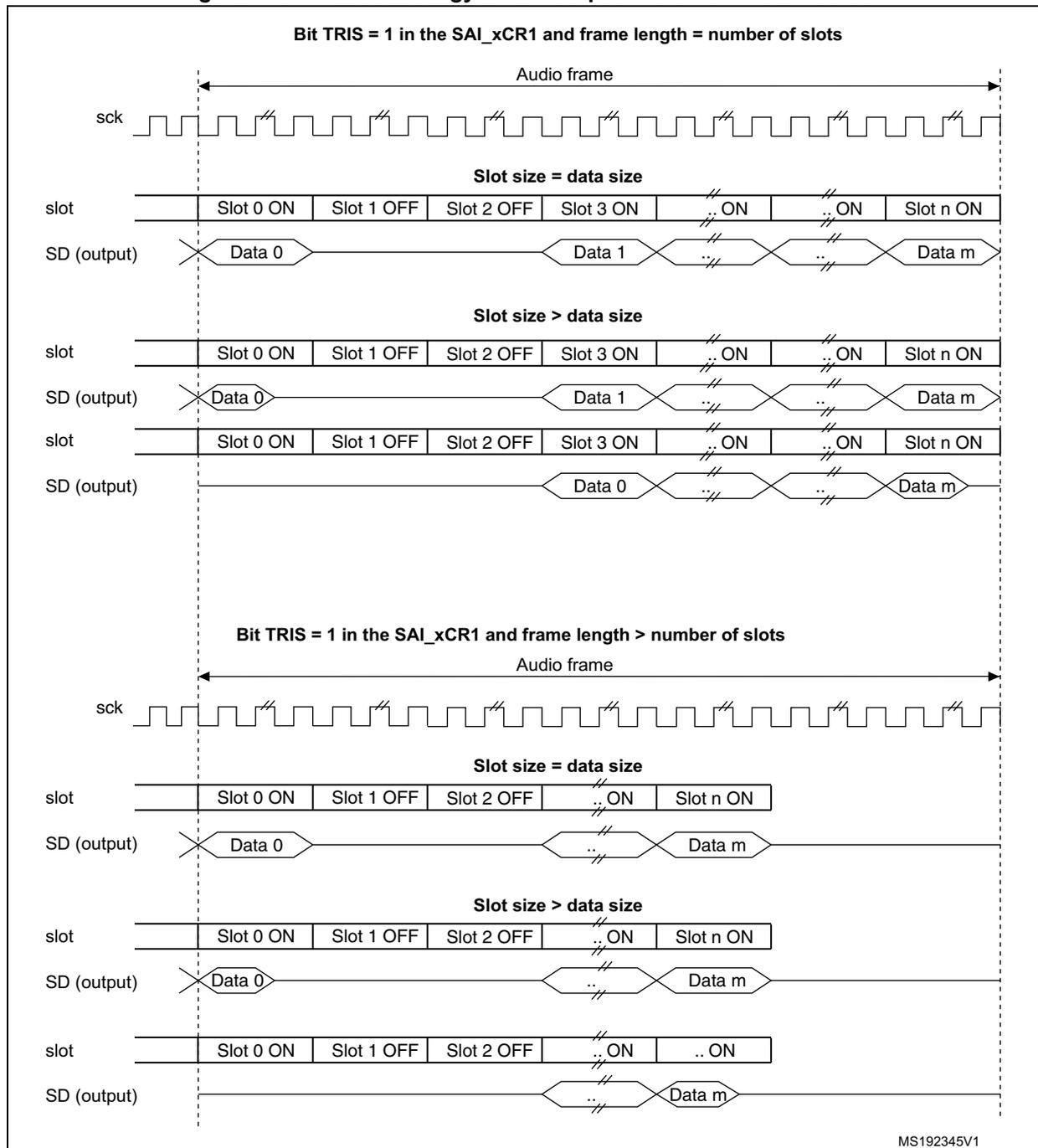
When the selected audio protocol uses the FS signal as a start of frame and a channel side identification (bit FSDEF = 1 in the SAI\_xFRCR register), the tristate mode is managed according to [Figure 420](#) (where bit TRIS in the SAI\_xCR1 register = 1, and FSDEF=1, and half frame length is higher than number of slots/2, and NBSLOT=6).
