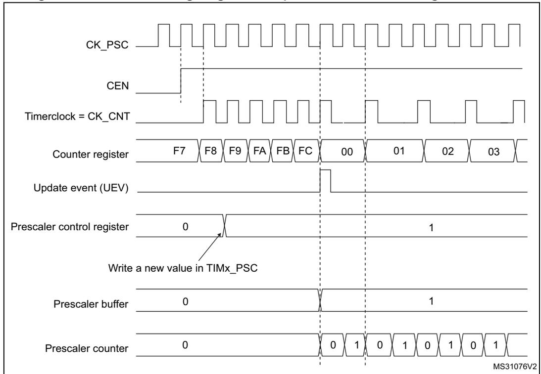
Figure 272. Counter timing diagram with prescaler division change from 1 to 4
