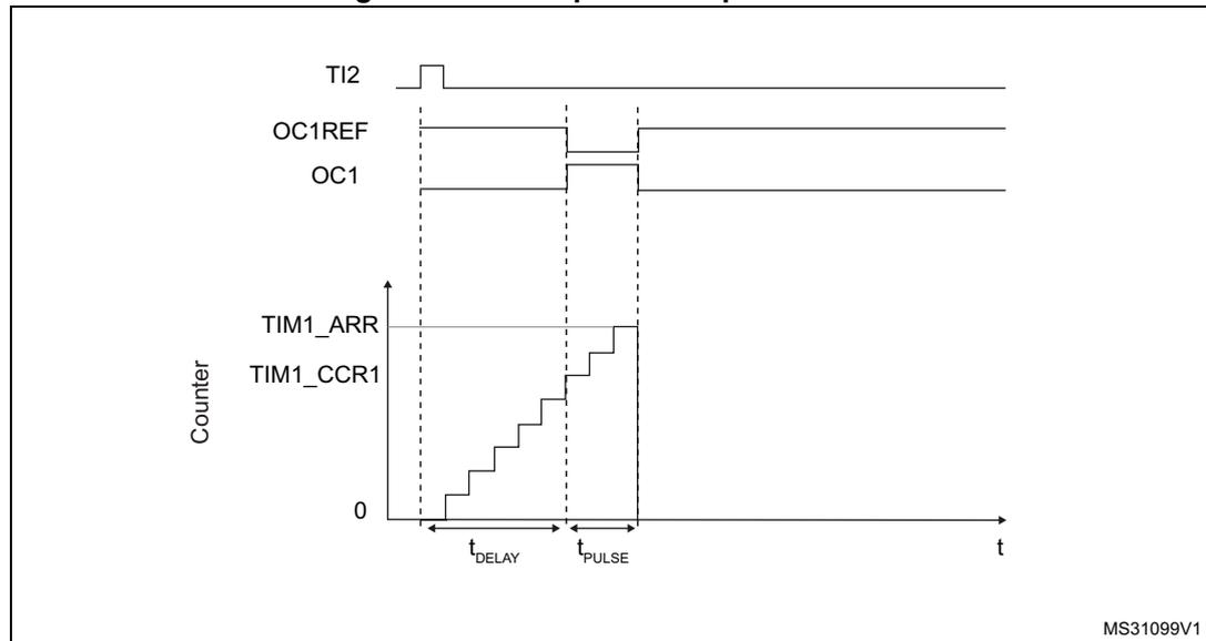
For example you may want to generate a positive pulse on OC1 with a length of  $t_{PULSE}$  and after a delay of  $t_{DELAY}$  as soon as a positive edge is detected on the TI2 input pin.
