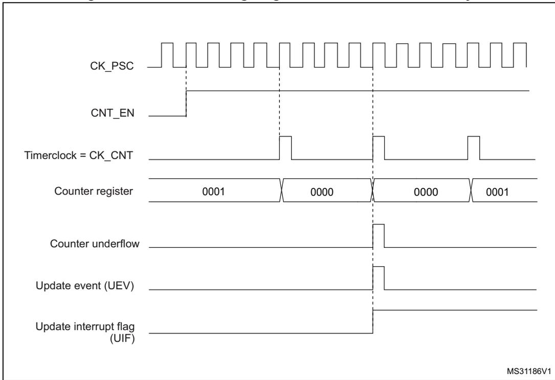
Figure 171. Counter timing diagram, internal clock divided by N
