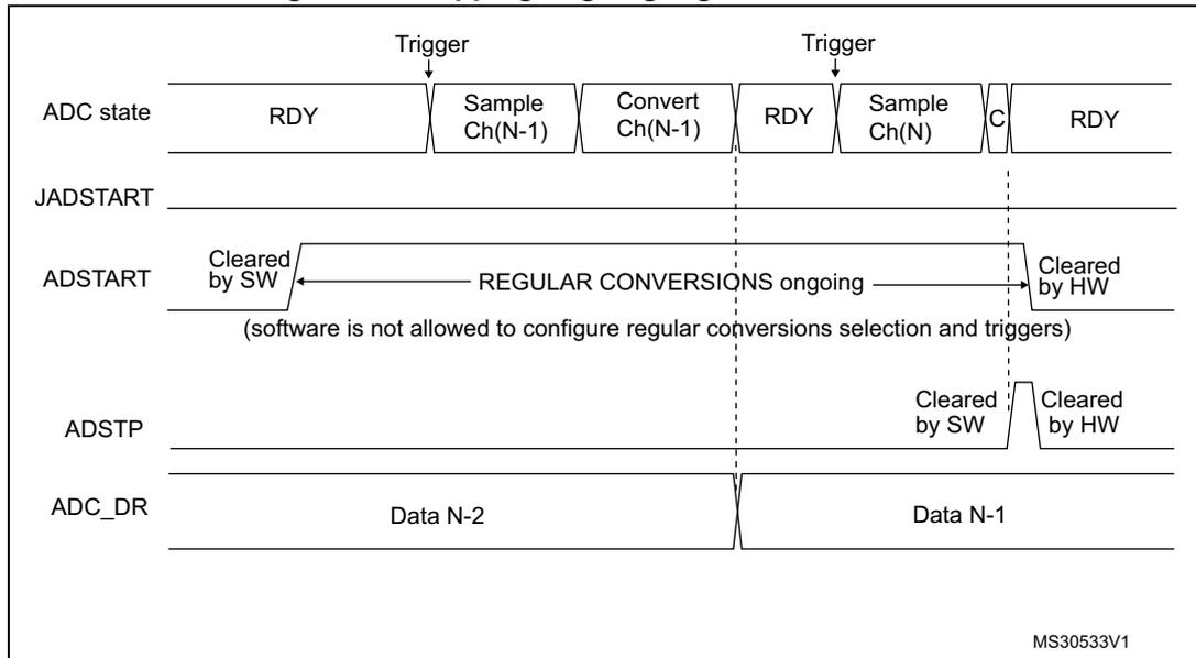
Figure 69. Stopping ongoing regular and injected conversions
