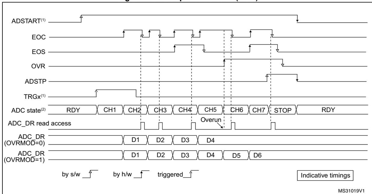
*Note:* There is no overrun detection on the injected channels since there is a dedicated data register for each of the four injected channels.
