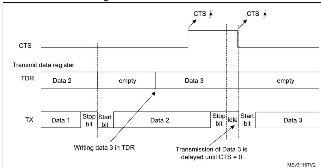
**Note:** For correct behavior, CTS must be asserted at least 3 LPUART clock source periods before the end of the current character. In addition it should be noted that the CTSCF flag may not be set for pulses shorter than 2 x PCLK periods.
