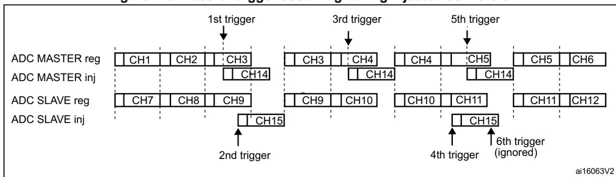
**Combined injected simultaneous plus interleaved**
