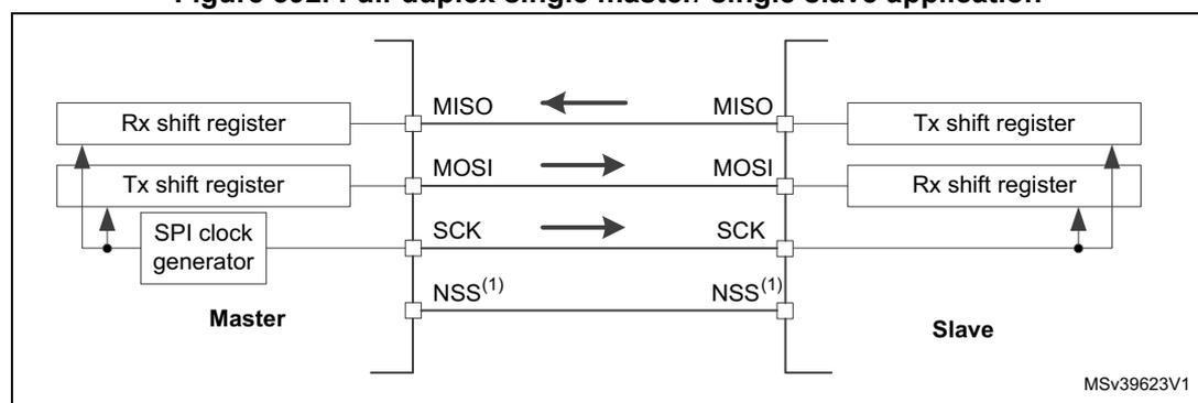
1. The NSS pins can be used to provide a hardware control flow between master and slave. Optionally, the pins can be left unused by the peripheral. Then the flow has to be handled internally for both master and slave. For more details see [Section 36.4.5: Slave select \(NSS\) pin management](#).
