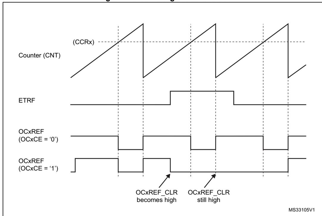
**Note:** In case of a PWM with a 100% duty cycle (if CCRx>ARR), OCxREF is enabled again at the next counter overflow.
