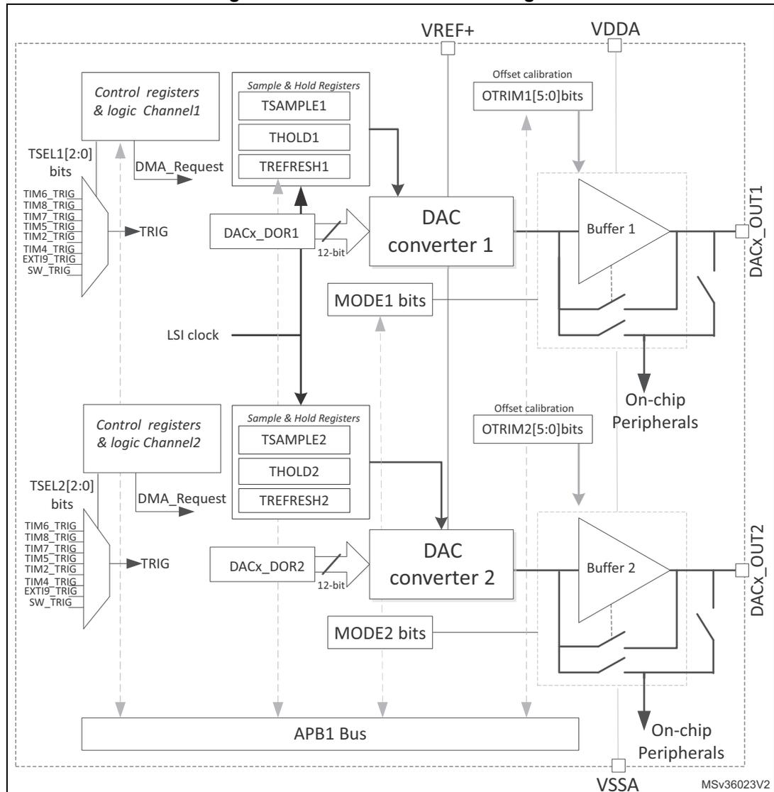
1. The output mode controller switch between the normal mode in buffer/unbuffer configuration and the sample&hold mode.
