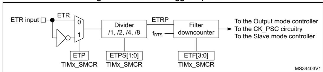
The ETR input comes from multiple sources: input pins (default configuration), comparator outputs and analog watchdogs. The selection is done with the ETRSEL[2:0] bitfield in the TIMx\_OR2 register and the TIMxOR1[1:0] and TIMxOR1[3:2] bitfields.
