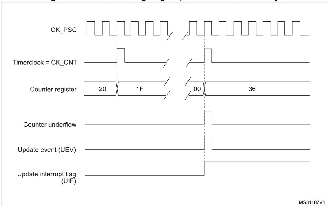
**Figure 172. Counter timing diagram, update event when repetition counter is not used**
