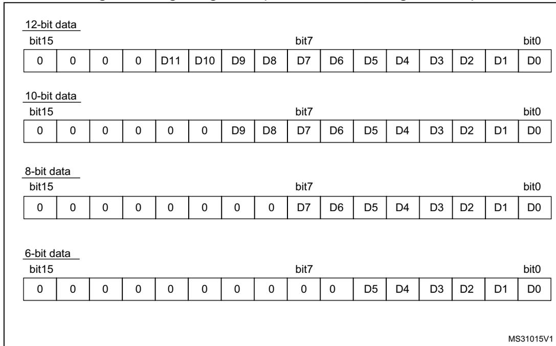
**Figure 89. Right alignment (offset enabled, signed value)**
