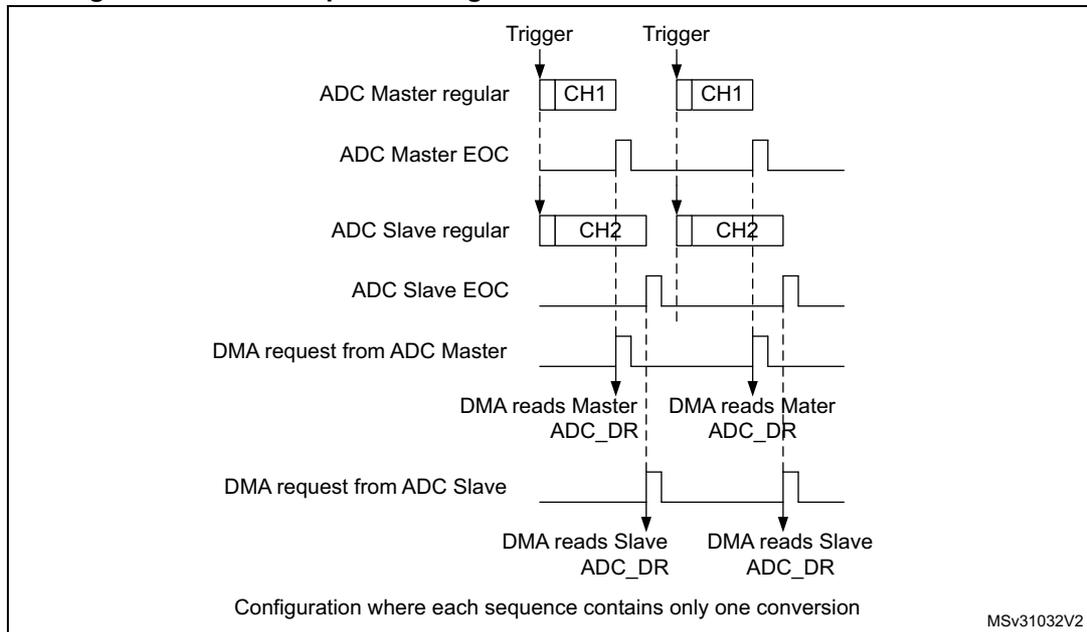
In simultaneous regular and interleaved modes, it is also possible to save one DMA channel and transfer both data using a single DMA channel. For this MDMA bits must be configured in the ADCx\_CCR register:
