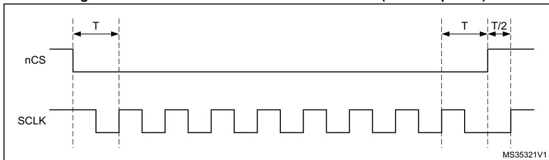
When the FIFO stays full in a read operation or if the FIFO stays empty in a write operation, the operation stalls and CLK stays low until firmware services the FIFO. If an abort occurs when an operation is stalled, nCS rises just after the abort is requested and then CLK rises one half of a CLK cycle later, as shown in [Figure 57](#).
