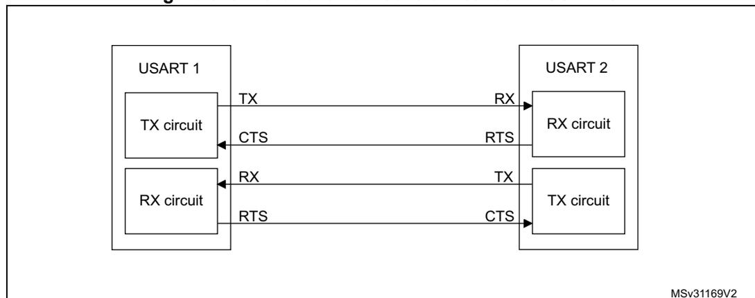
RS232 RTS and CTS flow control can be enabled independently by writing the RTSE and CTSE bits respectively to 1 (in the USARTx\_CR3 register).
