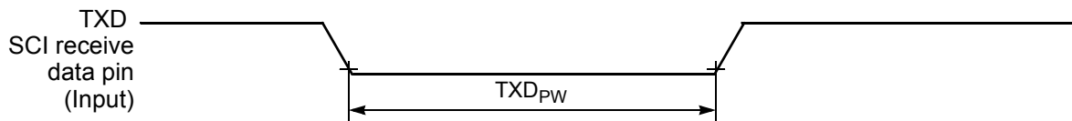
Figure 10-17 TXD Pulse Width
