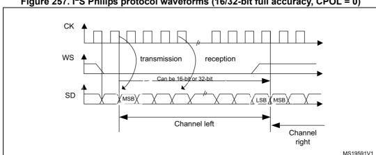
Figure 257. I<sup>2</sup>S Philips protocol waveforms (16/32-bit full accuracy, CPOL = 0)
