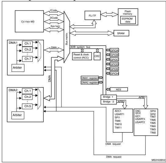
Figure 35. DMA block diagram in Cat.3 STM32L1xxxx devices
