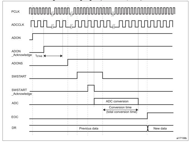
Figure 41. Timing diagram (normal mode, PDI=0)
