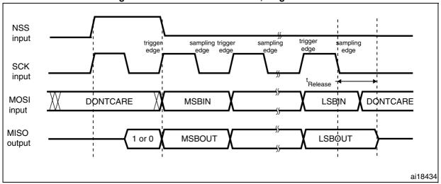
Figure 243. TI mode - Slave mode, single transfer
