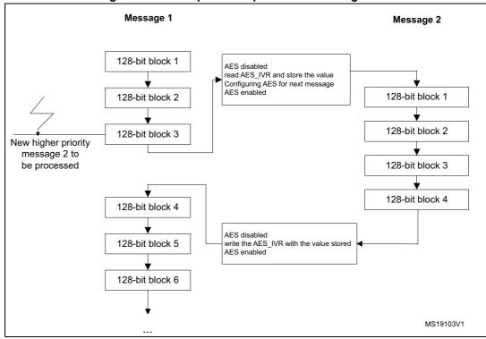
Figure 174. Example of suspend mode management
