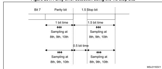
Figure 231. Parity error detection using the 1.5 stop bits
