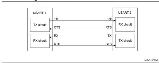
Figure 236. Hardware flow control between 2 USARTs
