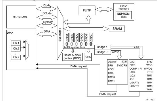
Figure 1. System architecture (Cat.1 and Cat.2 devices)
