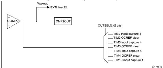
Figure 67. Redirecting the COMP2 output
