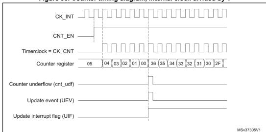
Figure 93. Counter timing diagram, internal clock divided by 1
