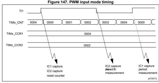
The PWM input mode can be used only with the TIMx\_CH1/TIMx\_CH2 signals due to the fact that only TI1FP1 and TI2FP2 are connected to the slave mode controller.
