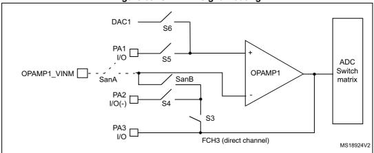
The routing for the three operational amplifiers can be selected by OPAMP\_CSR register.
