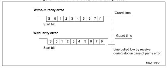
Figure 230. ISO 7816-3 asynchronous protocol
