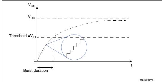
Figure 30. Sampling capacitor charge overview
