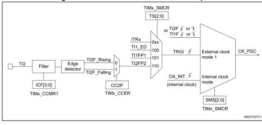
Figure 142. TI2 external clock connection example
