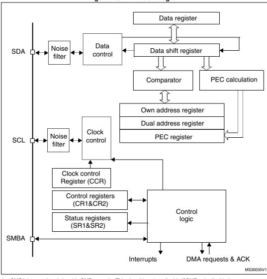
Figure 209. I<sup>2</sup>C block diagram
