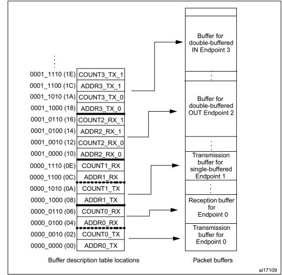
Figure 187. Packet buffer areas with examples of buffer description table locations
