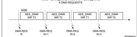
Figure 185. DMA requests during Output phase (AES\_OUT)
