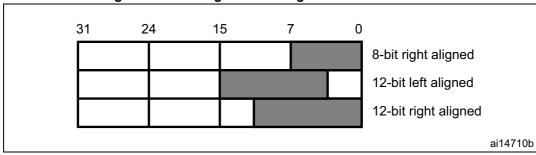
Figure 56. Data registers in single DAC channel mode
