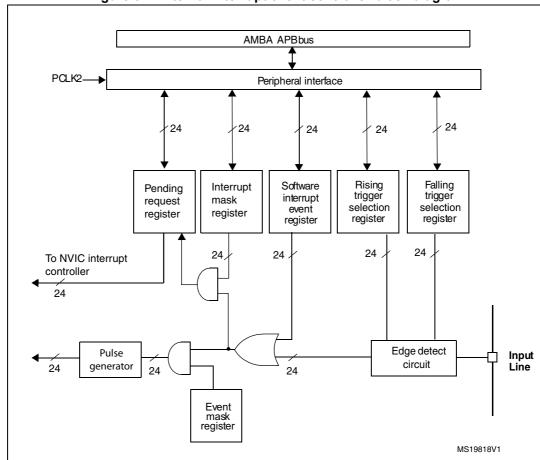
Figure 32. External interrupt/event controller block diagram
