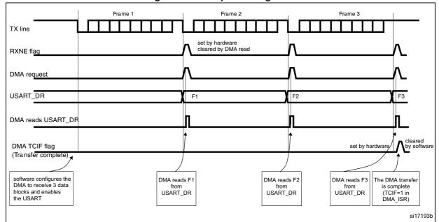
Figure 235. Reception using DMA
