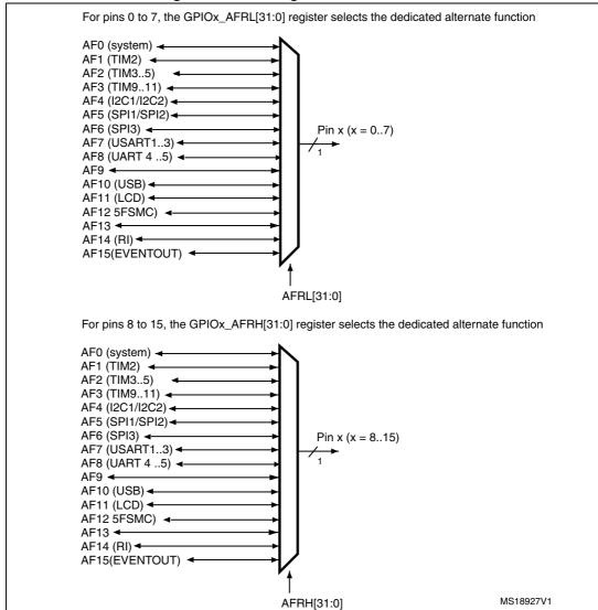
Figure 20. Selecting an alternate function
