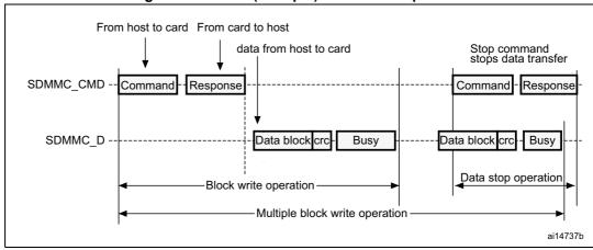
Figure 278. SDIO (multiple) block write operation
