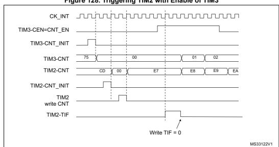
Figure 128. Triggering TIM2 with Enable of TIM3
