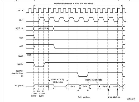
Figure 206. Synchronous multiplexed read mode - NOR, PSRAM (CRAM)
