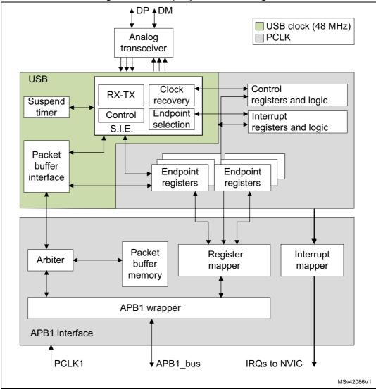
Figure 186. USB peripheral block diagram
