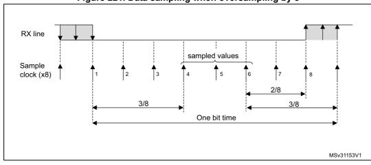
Figure 221. Data sampling when oversampling by 8
