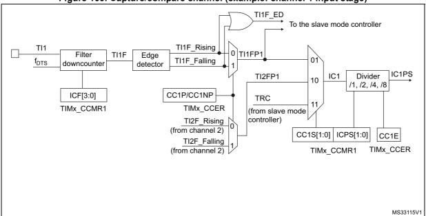
Figure 109. Capture/compare channel (example: channel 1 input stage)
