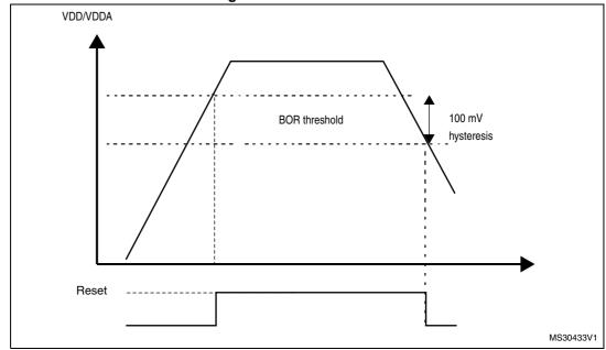
Figure 12. BOR thresholds
