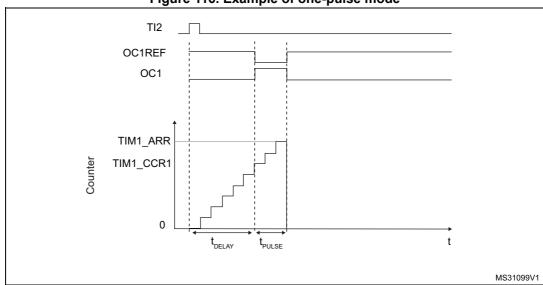
Figure 116. Example of one-pulse mode
