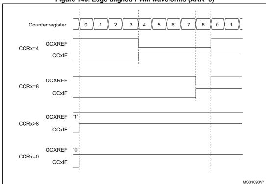
Figure 149. Edge-aligned PWM waveforms (ARR=8)
