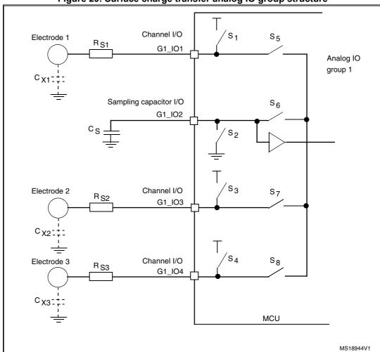
Figure 29. Surface charge transfer analog IO group structure
