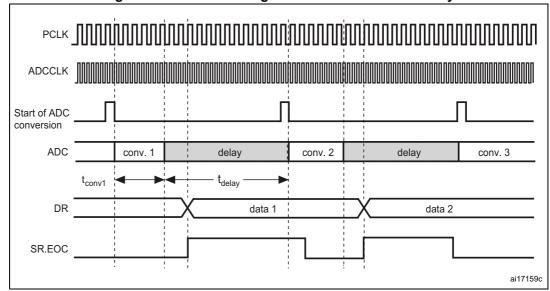
Figure 48. Continuous regular conversions with a delay
