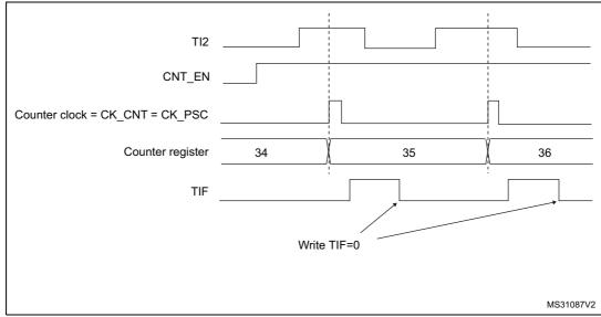
Figure 106. Control circuit in external clock mode 1
