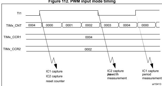
Figure 112. PWM input mode timing
