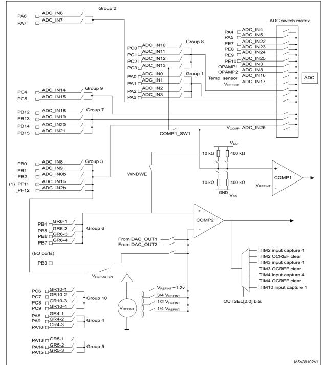
Figure 26. Routing interface (RI) block diagram for Cat.3 devices
