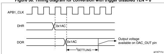
Figure 58. Timing diagram for conversion with trigger disabled TEN = 0
