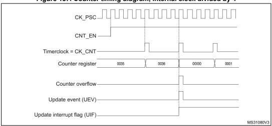
Figure 138. Counter timing diagram, internal clock divided by N
