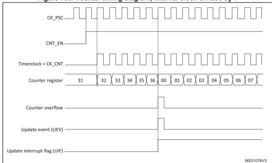
Figure 135. Counter timing diagram, internal clock divided by 1
