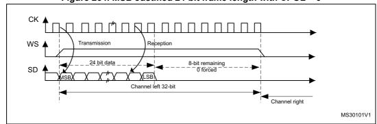
Figure 264. MSB Justified 24-bit frame length with CPOL = 0
