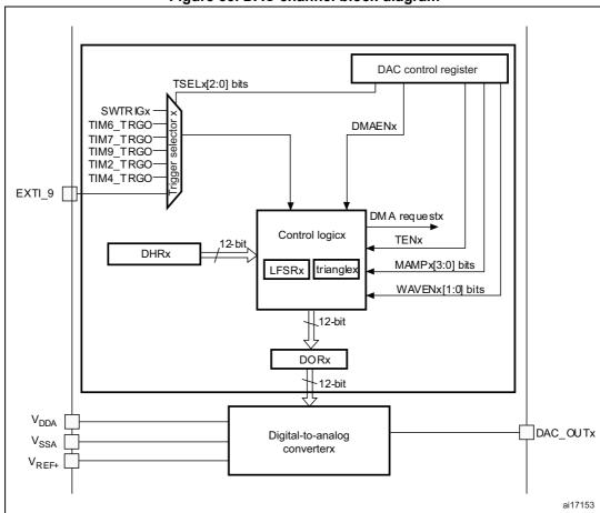
Figure 55. DAC channel block diagram
