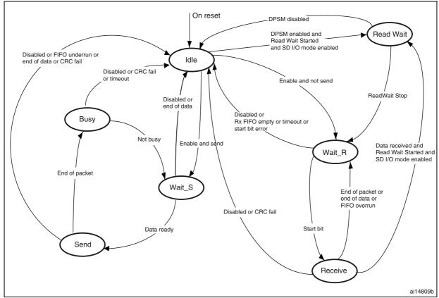
Figure 288. Data path state machine (DPSM)
