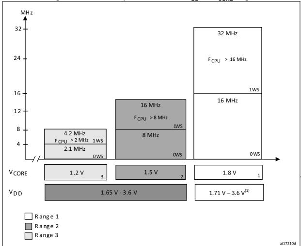
Figure 9. STM32L1xxxx performance versus V<sub>DD</sub> and V<sub>CORE</sub> range
