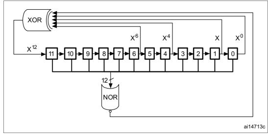
Figure 59. DAC LFSR register calculation algorithm
