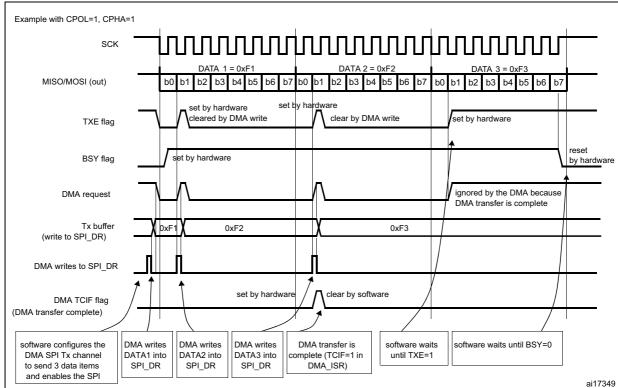
Figure 253. Transmission using DMA
