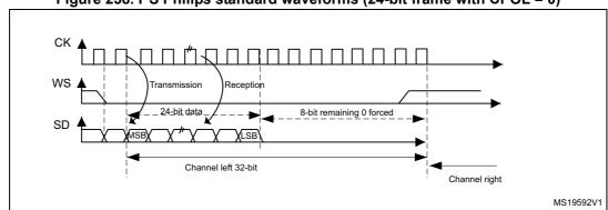
Figure 258. I<sup>2</sup>S Philips standard waveforms (24-bit frame with CPOL = 0)
