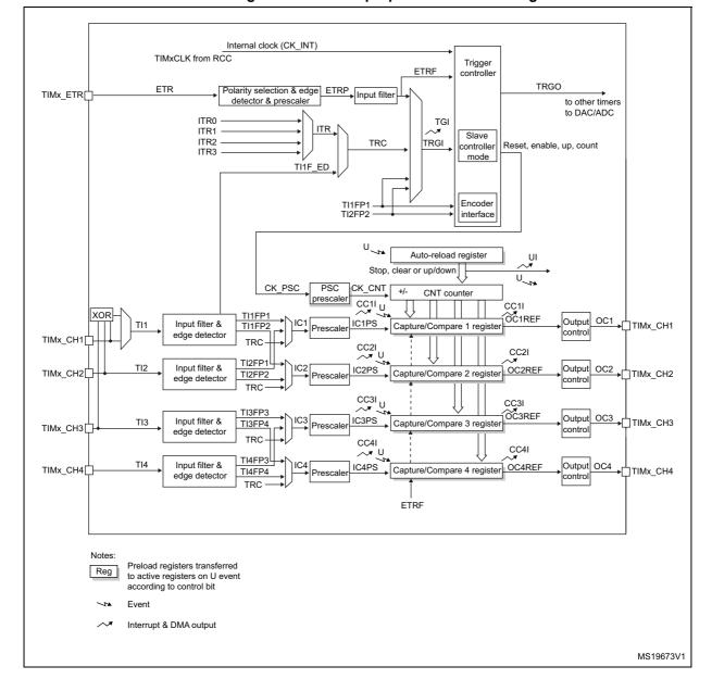
Figure 84. General-purpose timer block diagram
