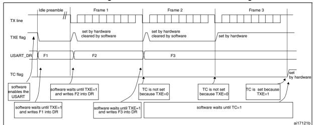
Figure 218. TC/TXE behavior when transmitting
