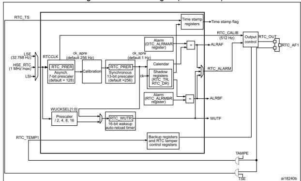
Figure 164. RTC block diagram (Cat.1 devices)
