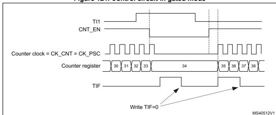
Figure 121. Control circuit in gated mode
