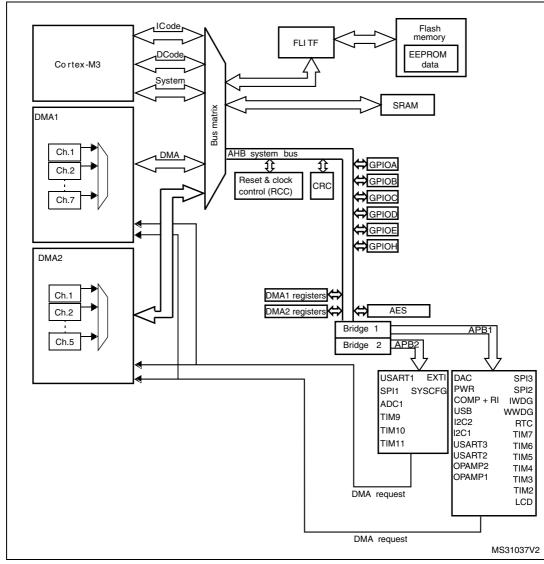
Figure 2. System architecture (Cat.3 devices)
