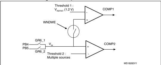
To use the COMP1 and COMP2 comparators in window mode, the application has to perform the following steps:
