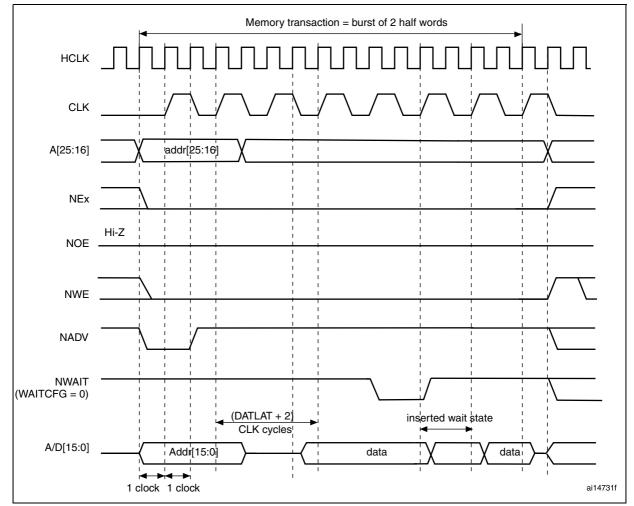
Figure 207. Synchronous multiplexed write mode - PSRAM (CRAM)
