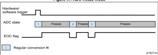
Figure 47. ADC freeze mode
