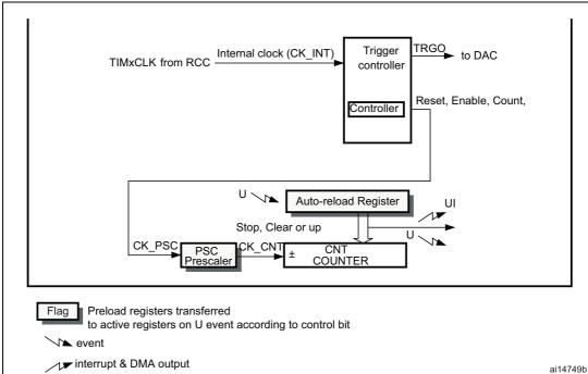
Figure 154. Basic timer block diagram
