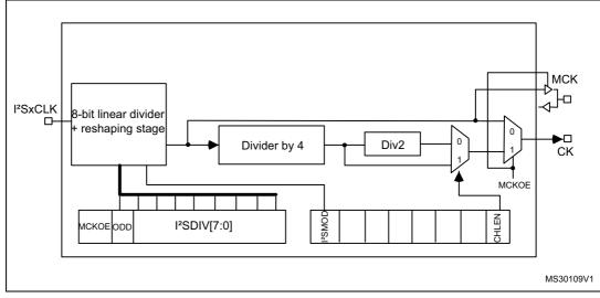
Figure 275. I<sup>2</sup>S clock generator architecture
