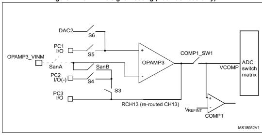
Figure 71. OPAMP3 signal routing (Cat.4 devices only)
