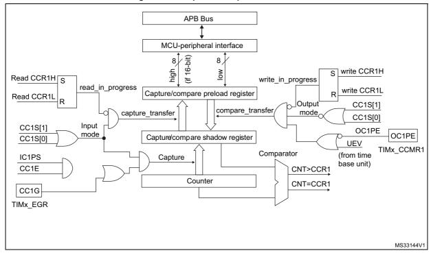
Figure 110. Capture/compare channel 1 main circuit
