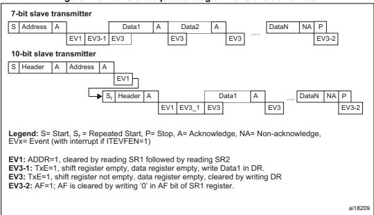
Figure 210. Transfer sequence diagram for slave transmitter
