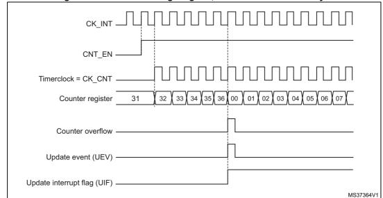
Figure 157. Counter timing diagram, internal clock divided by 1
