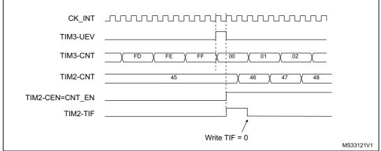
As in the previous example, both counters can be initialized before starting counting. Figure 128 shows the behavior with the same configuration as in Figure 127 but in trigger mode instead of gated mode (SMS=110 in the TIM2 SMCR register).
