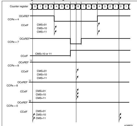
Figure 115. Center-aligned PWM waveforms (ARR=8)
