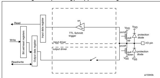
Figure 21. Input floating/pull up/pull down configurations
