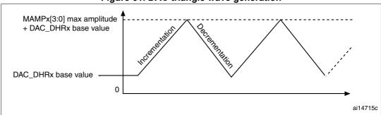
Figure 61. DAC triangle wave generation
