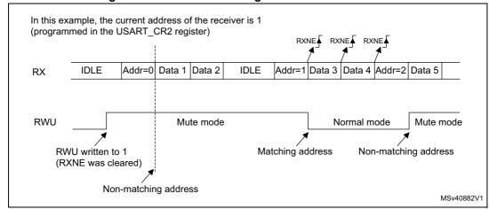
Figure 223. Mute mode using address mark detection
