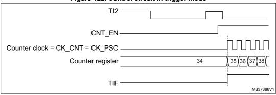
Figure 122. Control circuit in trigger mode
