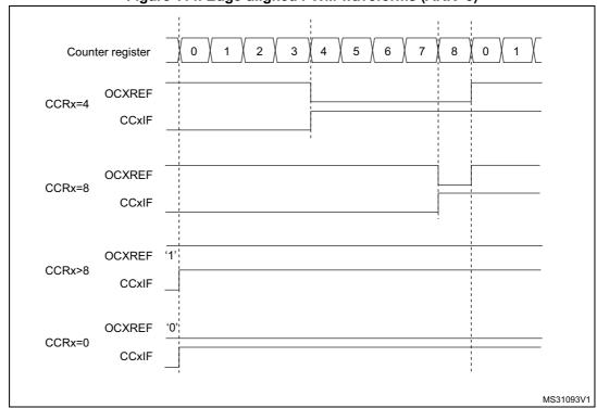
Figure 114. Edge-aligned PWM waveforms (ARR=8)
