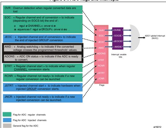
Figure 54. ADC flags and interrupts
