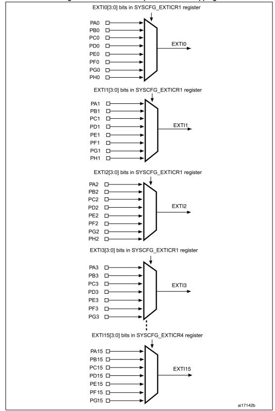
Figure 33. External interrupt/event GPIO mapping
