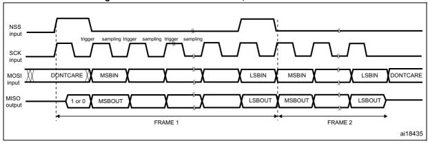
Figure 244. TI mode - Slave mode, continuous transfer
