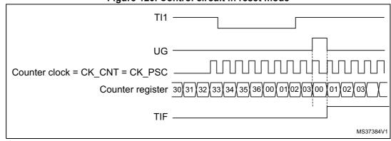
Figure 120. Control circuit in reset mode
