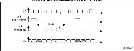
Figure 272. PCM standard waveforms (16-bit)
