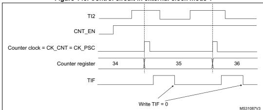
Figure 143. Control circuit in external clock mode 1
