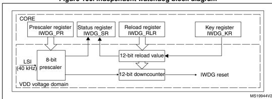
Figure 166. Independent watchdog block diagram
