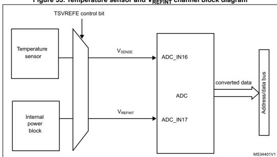
Figure 53. Temperature sensor and  $V_{REFINT}$  channel block diagram
