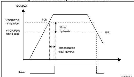
Figure 11. Power on reset/power down reset waveform
