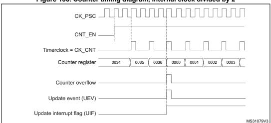
Figure 136. Counter timing diagram, internal clock divided by 2
