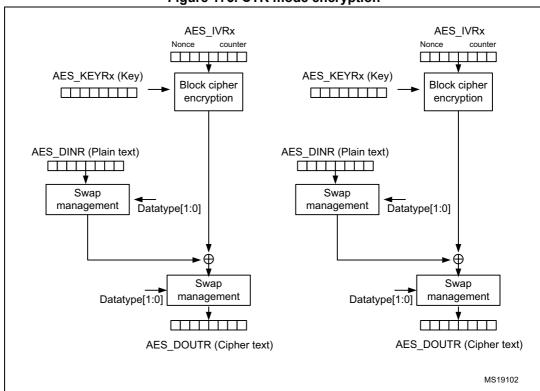
Figure 175. CTR mode encryption
