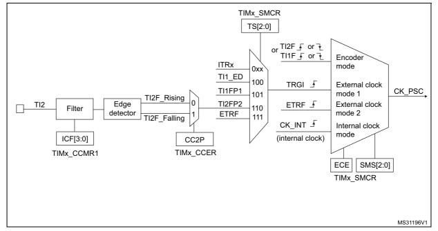
Figure 105. TI2 external clock connection example
