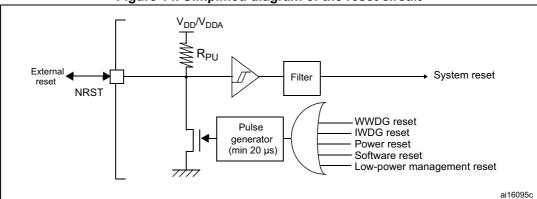
Figure 14. Simplified diagram of the reset circuit
