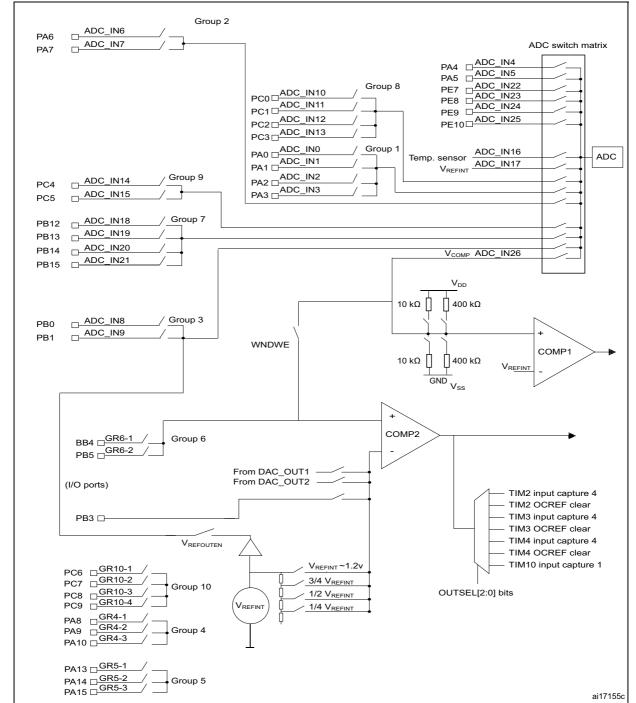
Figure 25. Routing interface (RI) block diagram for Cat.1 and Cat.2 devices
