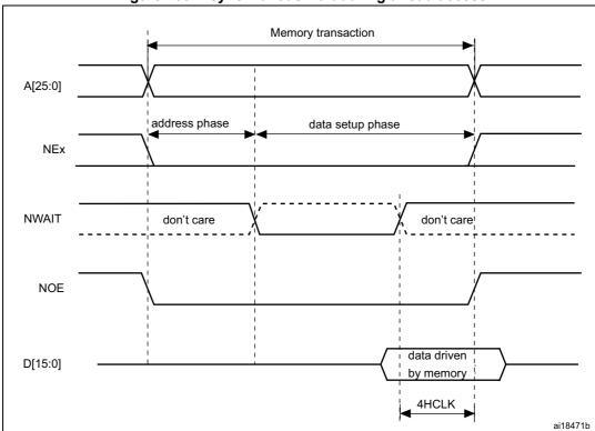
Figure 203. Asynchronous wait during a read access
