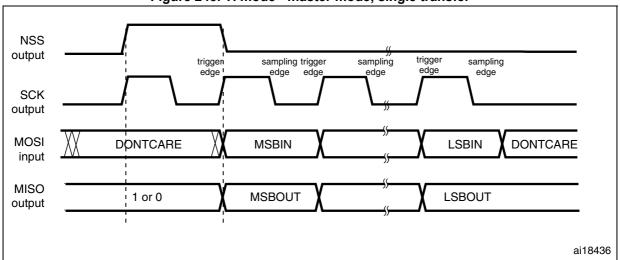
Figure 245. TI mode - master mode, single transfer
