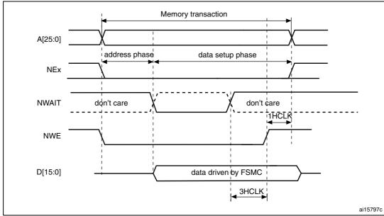
Figure 204. Asynchronous wait during a write access
