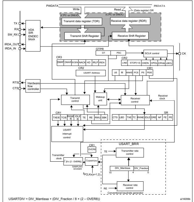
Figure 215. USART block diagram
