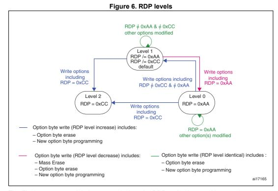
The Flash memory module is protected when the RDP option byte and its complement contain the following pair of values:
