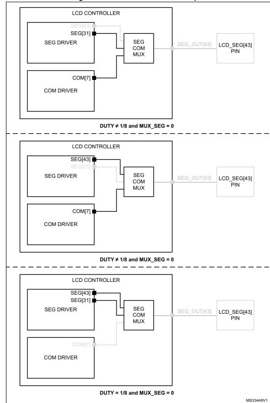
Figure 82. SEG/COM mux feature example
