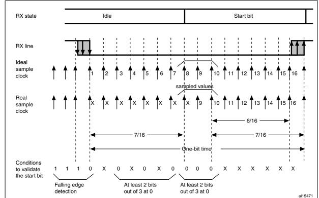
Figure 219. Start bit detection when oversampling by 16 or 8
