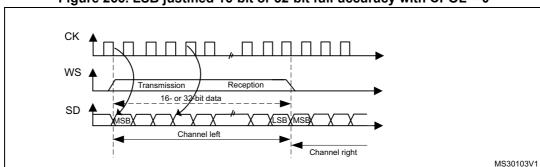
Figure 266. LSB justified 16-bit or 32-bit full-accuracy with CPOL = 0
