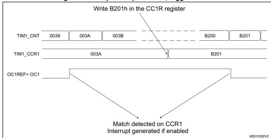
Figure 148. Output compare mode, toggle on OC1.
