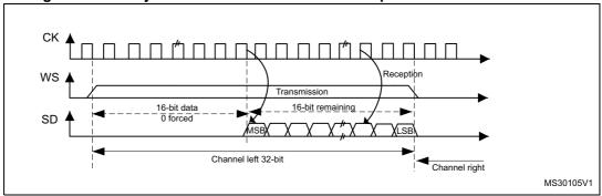
When 16-bit data frame extended to 32-bit channel frame is selected during the I<sup>2</sup>S configuration phase, Only one access to SPI\_DR is required. The 16 remaining bits are forced by hardware to 0x0000 to extend the data to 32-bit format. In this case it corresponds to the half-word MSB.
