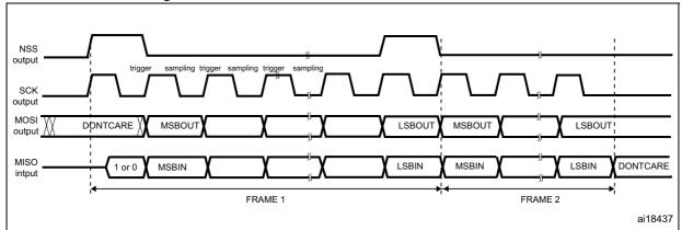
Figure 246. TI mode - master mode, continuous transfer
