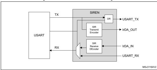
Figure 232. IrDA SIR ENDEC- block diagram
