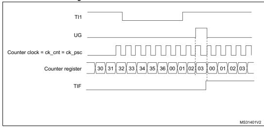
Figure 151. Control circuit in reset mode
