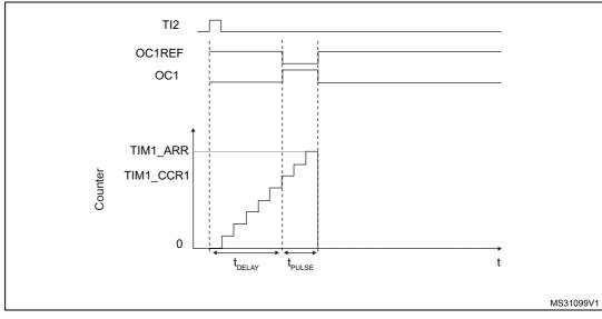
Figure 150. Example of one pulse mode.
