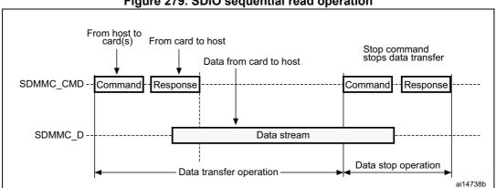
Figure 279. SDIO sequential read operation
