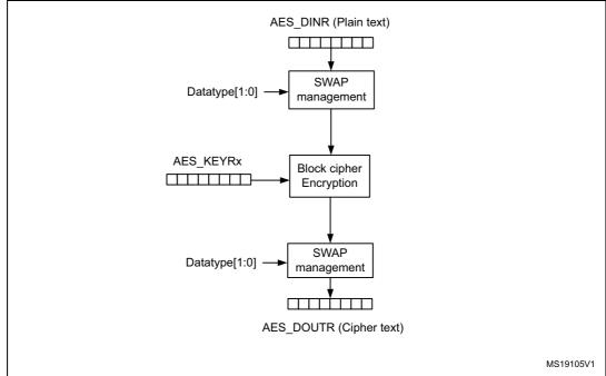
Figure 170. ECB encryption mode
