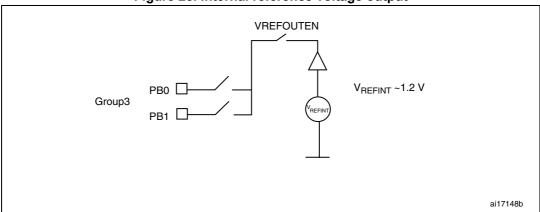
The V<sub>REFINT</sub> output can be routed to any I/O in group 3 by following this procedure:
