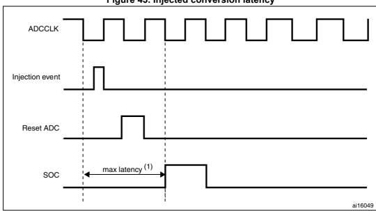
Figure 43. Injected conversion latency
