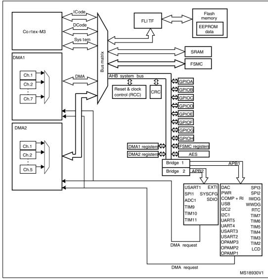
Figure 3. System architecture (Cat.4 devices)
