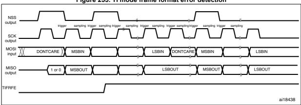
Figure 255. TI mode frame format error detection
