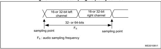
Figure 274. Audio sampling frequency definition
