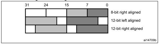
Figure 57. Data registers in dual DAC channel mode
