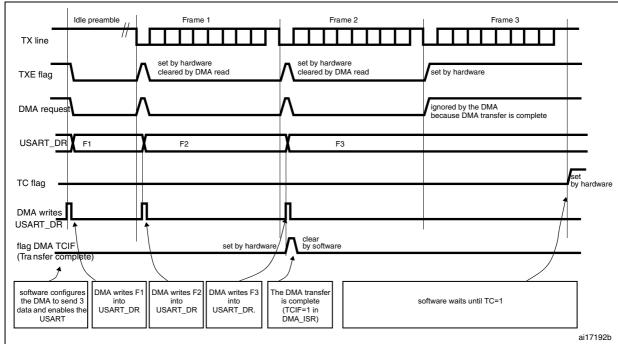
Figure 234. Transmission using DMA
