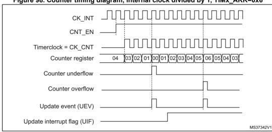
Figure 98. Counter timing diagram, internal clock divided by 1, TIMx\_ARR=0x6
