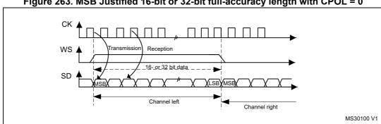
Figure 263. MSB Justified 16-bit or 32-bit full-accuracy length with CPOL = 0
