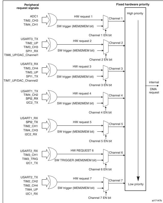
Figure 37. DMA1 request mapping
