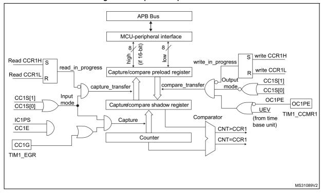
Figure 145. Capture/compare channel 1 main circuit
