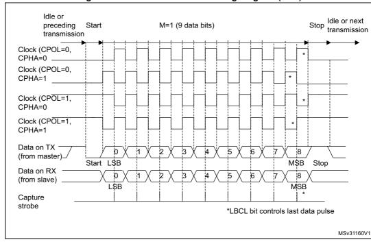
Figure 228. USART data clock timing diagram (M=1)
