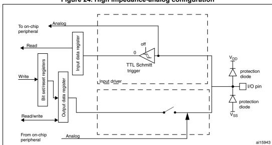
Figure 24. High impedance-analog configuration
