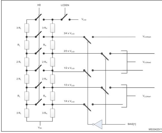
Figure 80. LCD voltage control
