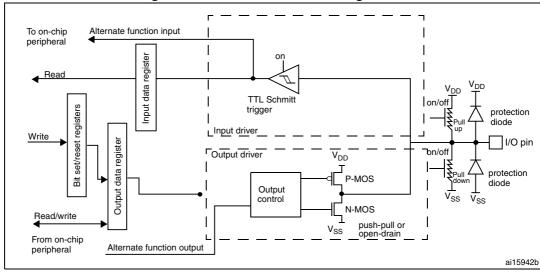
Figure 23. Alternate function configuration
