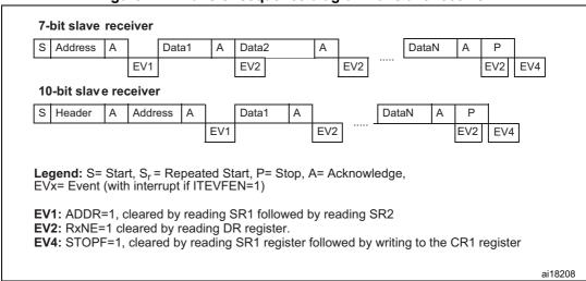
Figure 211. Transfer sequence diagram for slave receiver
