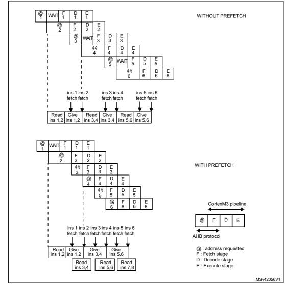
Figure 5. Sequential 32 bits instructions execution
