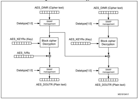
Note: When the AES is enabled, reading the AES\_IVR returns the value 0x00000000.
