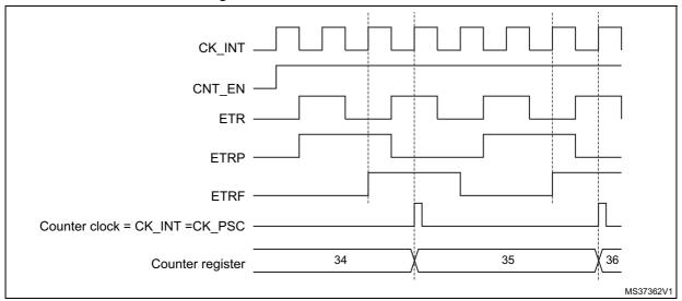
Figure 108. Control circuit in external clock mode 2
