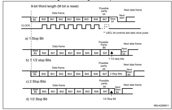
Figure 217. Configurable stop bits
