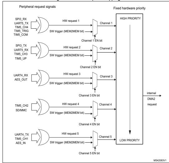
Figure 38. DMA2 request mapping
