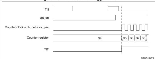
Figure 153. Control circuit in trigger mode
