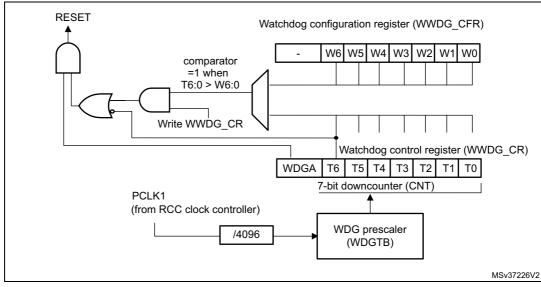
Figure 167. Watchdog block diagram
