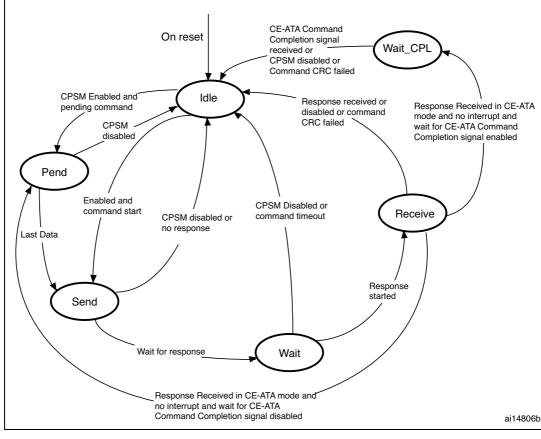
Figure 285. Command path state machine (CPSM)
