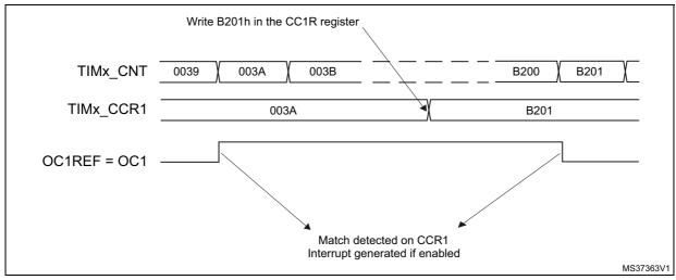
Figure 113. Output compare mode, toggle on OC1
