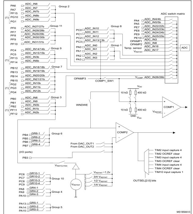
Figure 27. Routing interface (RI) block diagram for Cat.4, Cat.5 and Cat.6 devices
