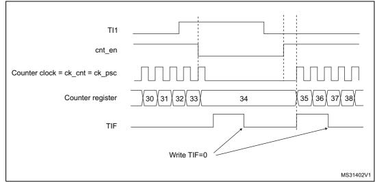
Figure 152. Control circuit in gated mode
