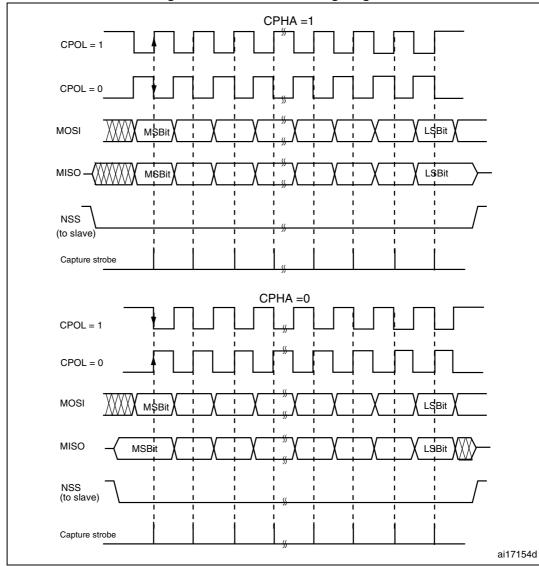
Figure 242. Data clock timing diagram
