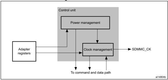
The control unit is illustrated in *Figure 283*. It consists of a power management subunit and a clock management subunit.
