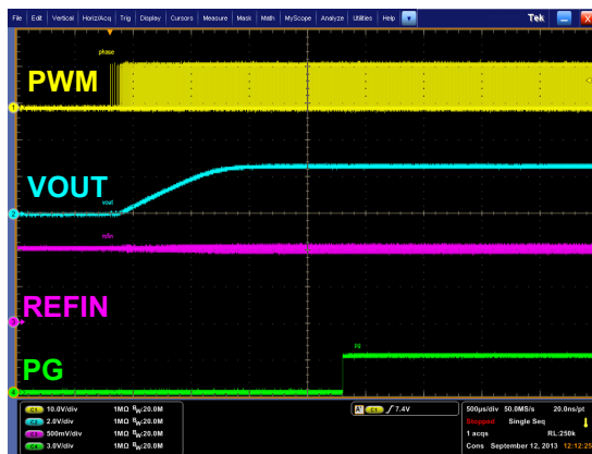
Figure 6. Soft-start with ext. ref. div. 2
