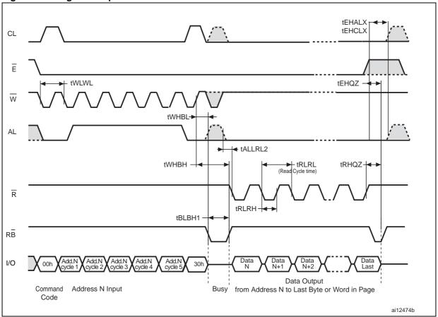
Figure 34. Page program AC waveform CL
