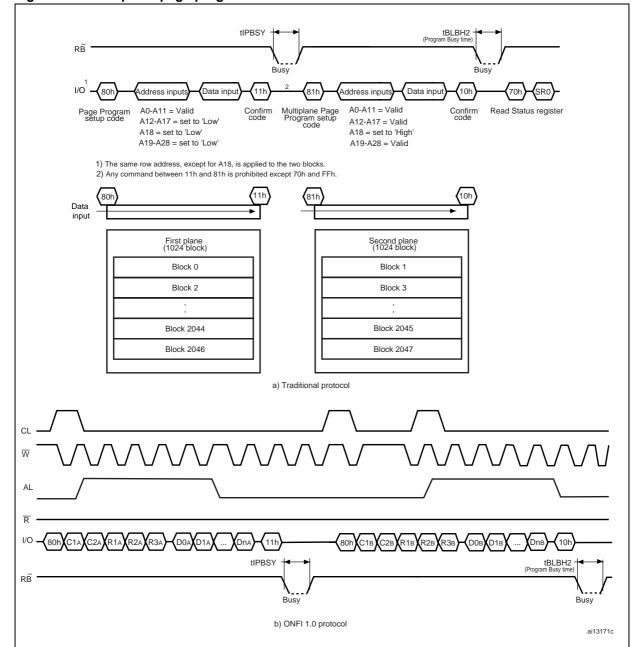
Figure 13. Multiplane page program waveform
