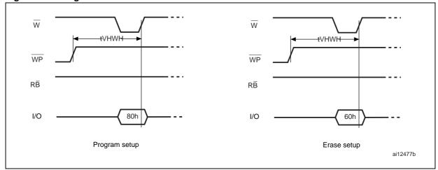
Figure 38. Program/erase disable waveform
