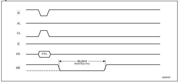
Figure 37. Program/erase enable waveform
