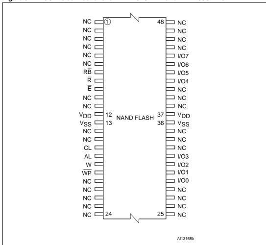
Figure 3. TSOP48 connections for NAND04G-B2D and NAND08G-BxC
