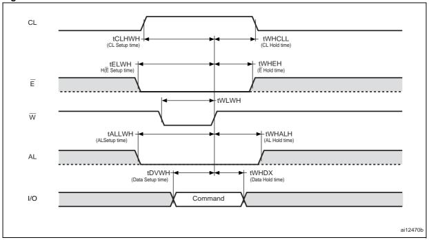
Figure 25. Address latch AC waveforms
