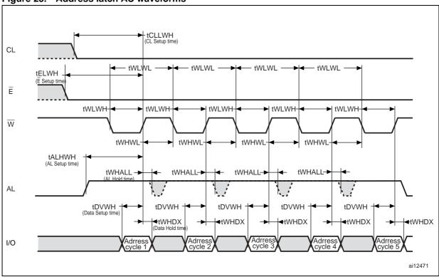
Figure 26. Data input latch AC waveforms
