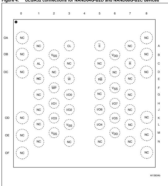
Figure 4. ULGA52 connections for NAND04G-B2D and NAND08G-B2C devices
