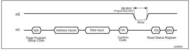
Figure 12. Random data input during sequential data input
