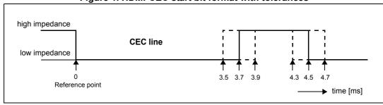
Figure 1. HDMI-CEC start bit format with tolerances
