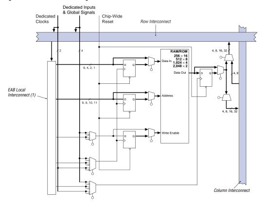
Figure 4. FLEX 10KE Device in Single-Port RAM Mode
