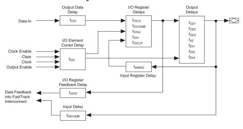
Figure 27. FLEX 10KE Device EAB Timing Model
