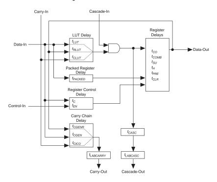
Figure 26. FLEX 10KE Device IOE Timing Model
