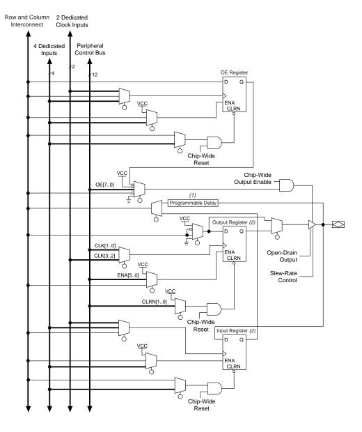
Figure 15. FLEX 10KE Bidirectional I/O Registers
