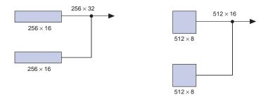
If necessary, all EABs in a device can be cascaded to form a single RAM block. EABs can be cascaded to form RAM blocks of up to 2,048 words without impacting timing. The Altera software automatically combines EABs to meet a designer's RAM specifications.
