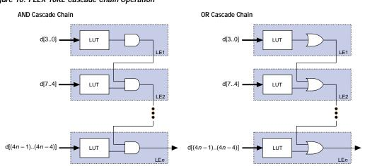
Figure 10. FLEX 10KE Cascade Chain Operation
