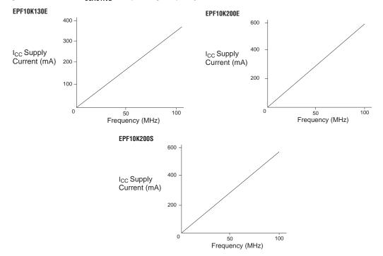
Figure 31. FLEX 10KE I<sub>CCACTIVE</sub> vs. Operating Frequency (Part 2 of 2)
