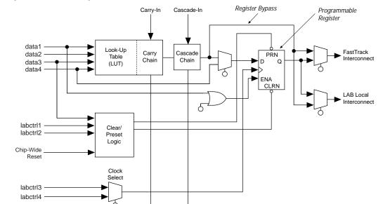
Figure 8. FLEX 10KE Logic Element
