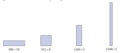
Larger blocks of RAM are created by combining multiple EABs. For example, two  $256\times16$  RAM blocks can be combined to form a  $256\times32$  block; two  $512\times8$  RAM blocks can be combined to form a  $512\times16$  block (see Figure 6).
