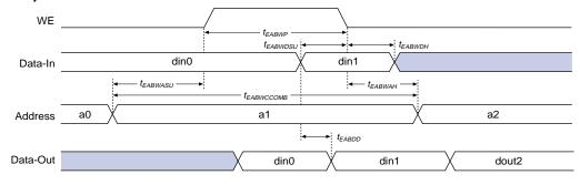
Figure 30. EAB Synchronous Timing Waveforms
