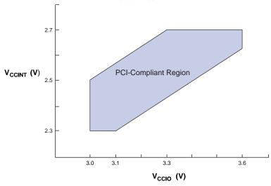
Figure 22. Relationship between  $V_{CCIO}$  &  $V_{CCINT}$  for 3.3-V PCI Compliance
