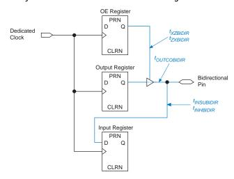
Figure 28. Synchronous Bidirectional Pin External Timing Model
