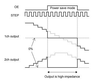
When the OE pin is set High, the output is forced OFF and goes to high impedance.
