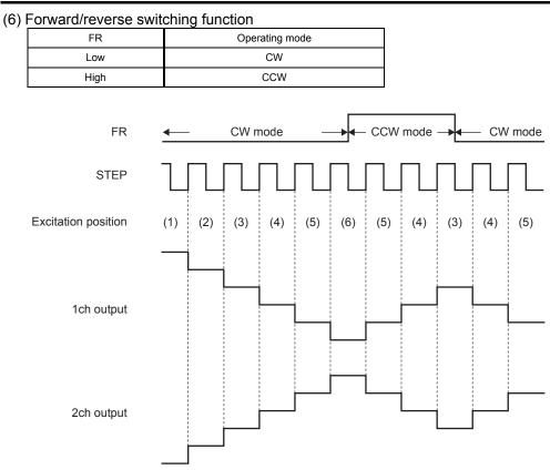
The internal D/A converter proceeds by one bit at the rising edge of the input STEP pulse. In addition, CW and CCW mode are switched by setting the FR pin. In CW mode, the channel 2 current phase is delayed by 90° relative to the channel 1 current. In CCW mode, the channel 2 current phase is advanced by 90° relative to the channel 1 current.
