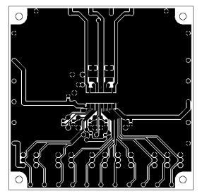
L1 : Copper wiring pattern diagram
