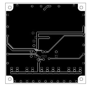
L2 : Copper wiring pattern diagram
