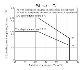
Substrate Specifications (Substrate recommended for operation of LV8746V)
