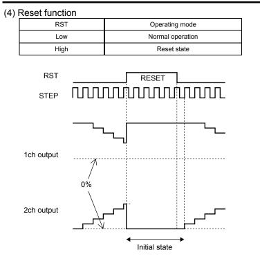
When the RST pin is set to High, the excitation position of the output is forcibly set to the initial state. When RST is then set to Low, the excitation position is advanced by the next STEP input.
