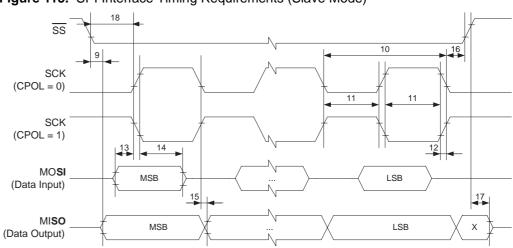
Figure 115. SPI Interface Timing Requirements (Slave Mode)
