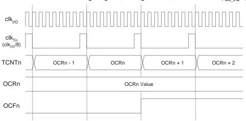
Figure 68. Timer/Counter Timing Diagram, Setting of OCF2, with Prescaler (f<sub>clk I/O</sub>/8)
