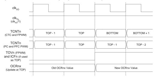
Figure 57. Timer/Counter Timing Diagram, no Prescaling
