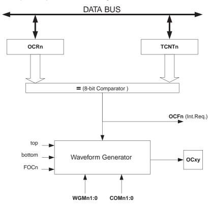
Figure 61. Output Compare Unit, Block Diagram
