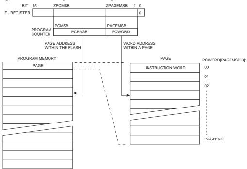
Figure 95. Addressing the Flash during SPM<sup>(1)</sup>
