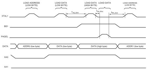
Note: 1. The timing requirements shown in Figure 102 (i.e., t<sub>DVXH</sub>, t<sub>XHXL</sub>, and t<sub>XLDX</sub>) also apply to loading operation.
