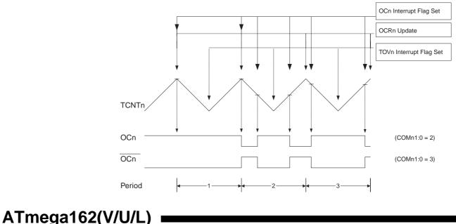
The Timer/Counter Overflow Flag (TOV2) is set each time the counter reaches BOT-TOM. The interrupt flag can be used to generate an interrupt each time the counter reaches the BOTTOM value.
