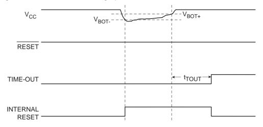
Figure 25. Brown-out Reset During Operation
