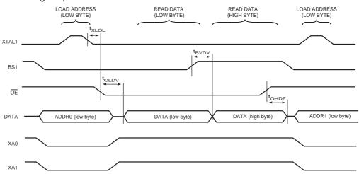
**Figure 104.** Parallel Programming Timing, Reading Sequence (within the Same Page) with Timing Requirements<sup>(1)</sup>
