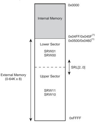
Note: 1. Address depends on the ATmega161 compability Fuse. See "SRAM Data Memory" on page 16 and Figure 9 on page 17 for details.
