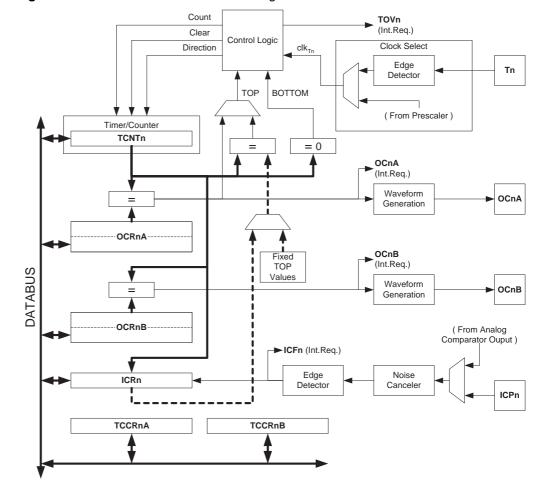
Figure 46. 16-bit Timer/Counter Block Diagram<sup>(1)</sup>
