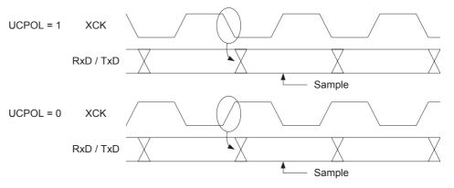
The UCPOL bit UCRSC selects which XCK clock edge is used for data sampling and which is used for data change. As Figure 77 shows, when UCPOL is zero the data will be changed at rising XCK edge and sampled at falling XCK edge. If UCPOL is set, the data will be changed at falling XCK edge and sampled at rising XCK edge.
