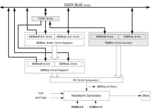
Figure 49. Output Compare Unit, Block Diagram
