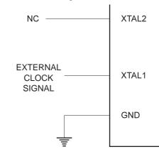
When this clock source is selected, start-up times are determined by the SUT Fuses as shown in Table 14.
