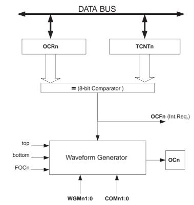
The OCR0 Register is double buffered when using any of the Pulse Width Modulation (PWM) modes. For the Normal and Clear Timer on Compare (CTC) modes of operation, the double buffering is disabled. The double buffering synchronizes the update of the OCR0 Compare Register to either top or bottom of the counting sequence. The synchronization prevents the occurrence of odd-length, non-symmetrical PWM pulses, thereby making the output glitch-free.
