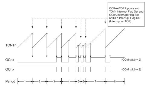
The Timer/Counter Overflow Flag (TOVn) is set each time the counter reaches TOP. In addition the OCnA or ICFn flag is set at the same timer clock cycle as TOVn is set when
