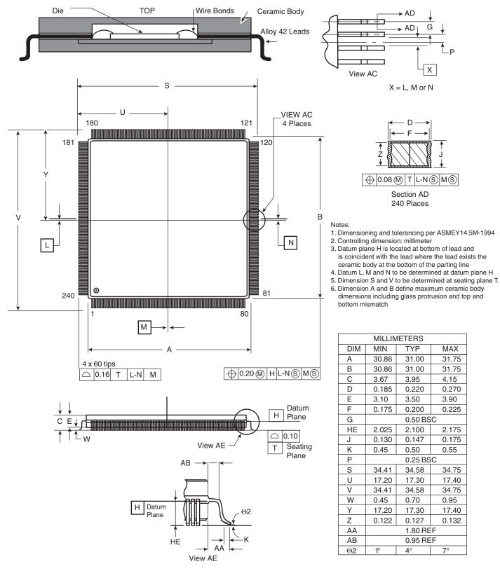
Figure 15-4. Mechanical Dimensions of the Wire-bond CERQUAD Package
