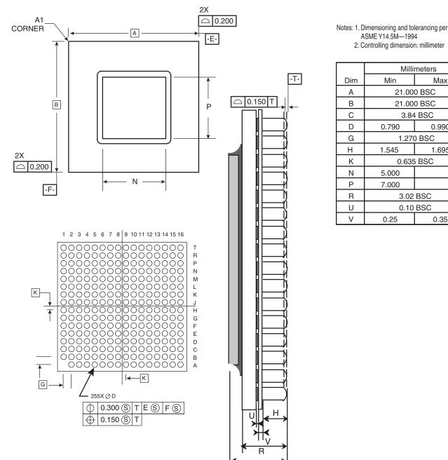
Figure 15-3. Mechanical Dimensions and Bottom Surface Nomenclature of the CI-CGA Package
