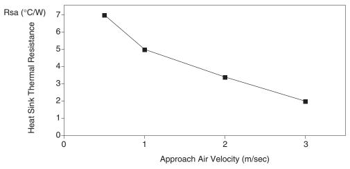
Assuming an air velocity of 1 m/sec, the associated overall thermal resistance and junction temperature, found in Table 8-1 will result.
