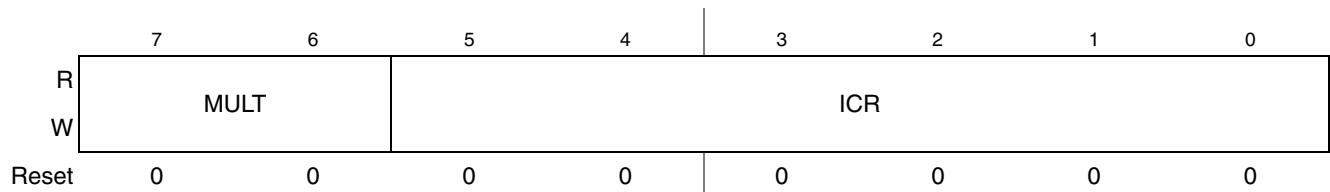
Figure 13-4. IIC Frequency Divider Register (IIC1F)
