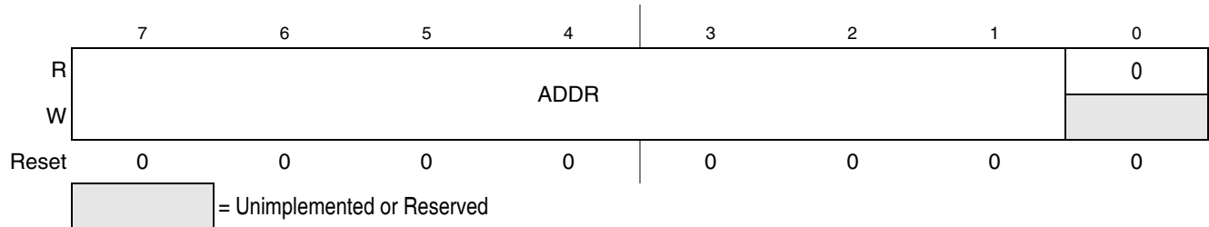
Figure 13-3. IIC Address Register (IIC1A)
